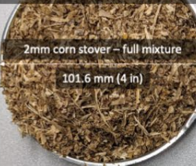
Air classified Size reduced to 2 mm
