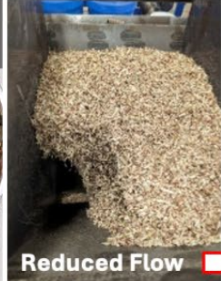
Air classified Size reduced to 4 mm
