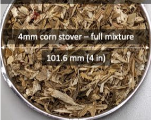
Air classified Size reduced to 4 mm
