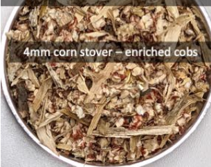
Air classified Size reduced to 4 mm
