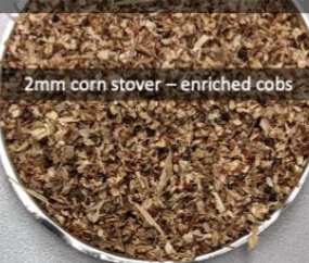
Air classified Size reduced to 2 mm
