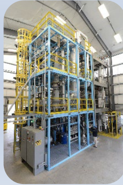
1 Ton / Day Pilot Scale Process Unit at RTI
