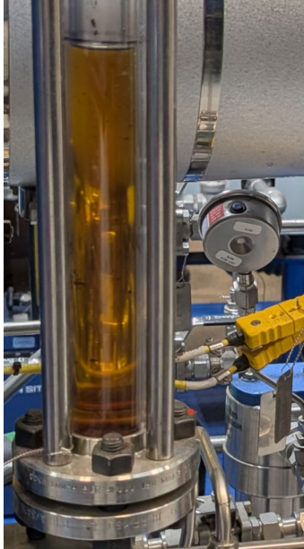
Scrubbing fluid (dodecane) after several runs
