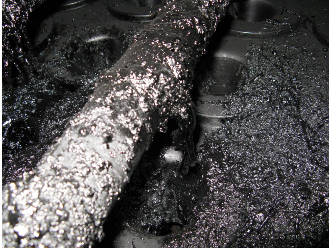
Tars from a conventional biomass gasifier
