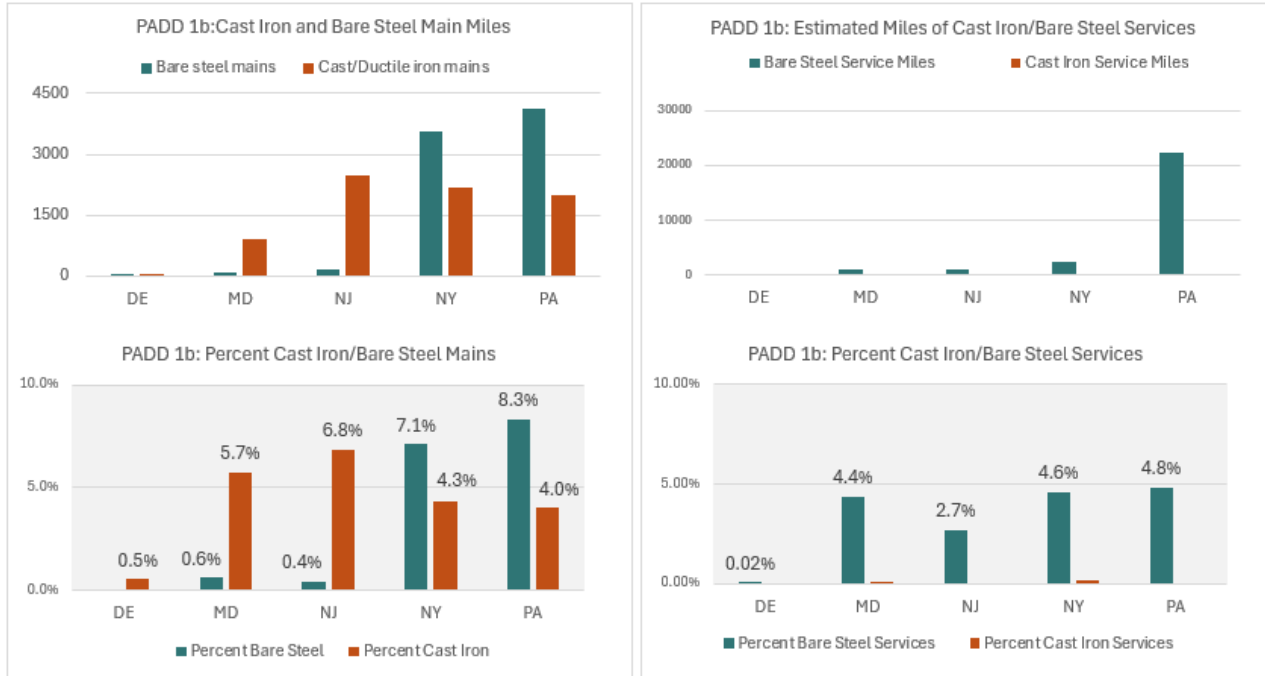
Figure 52. Summarized cast/ductile iron and bare steel distribution pipeline inventories in PADD 1b: Central Atlantic
