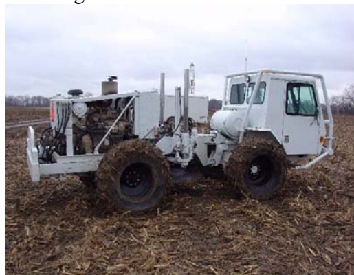
Figure 10.4. MiniVibe used in the Survey
