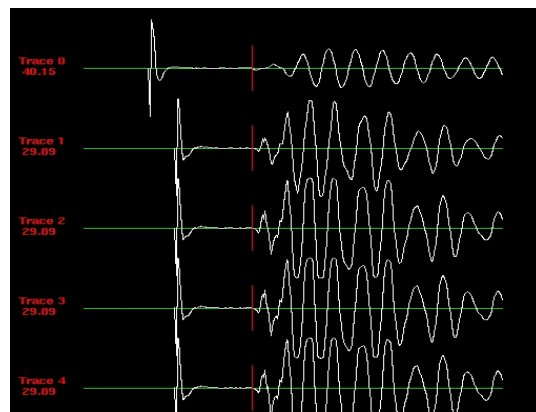
Figure 1. Travel time for a gas and water saturated coal sample
