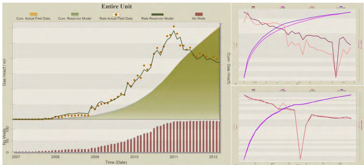
Figure 28: Entire Field History Matching Results and two wells as examples- Effect of Offset Well
