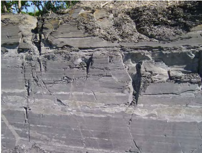
Figure 28. J1 fracture with calcite and pyrite cements on the surface. Plumose structure can be seen in the cement at right. Location: Wolfe Quarry, The Village at Union Springs, NY.
