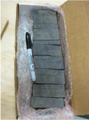
Figure 3: Marcellus shale core sample
