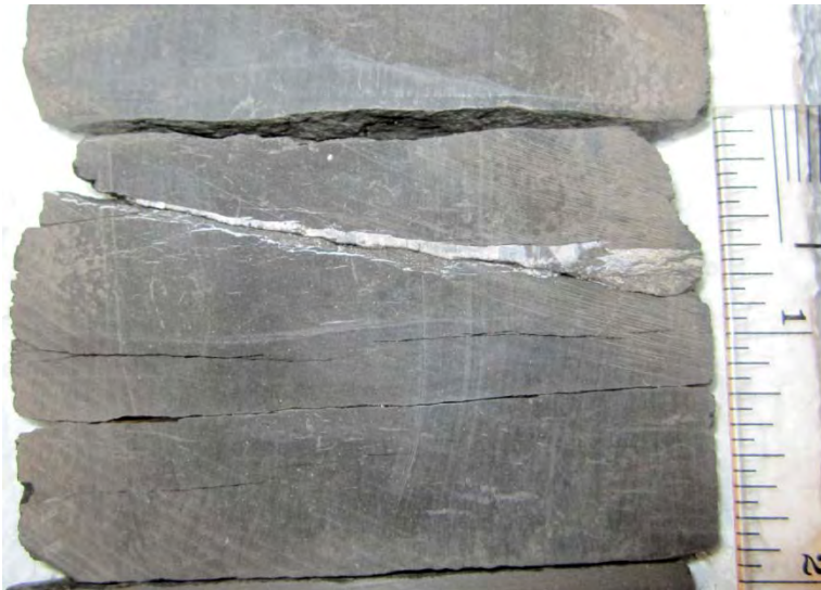
Figure 17. Low angle fracture at 6,567.6 ft.
