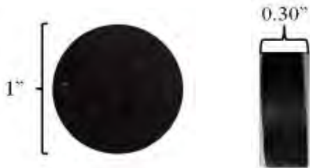
Figure 2: Core sample dimensions
