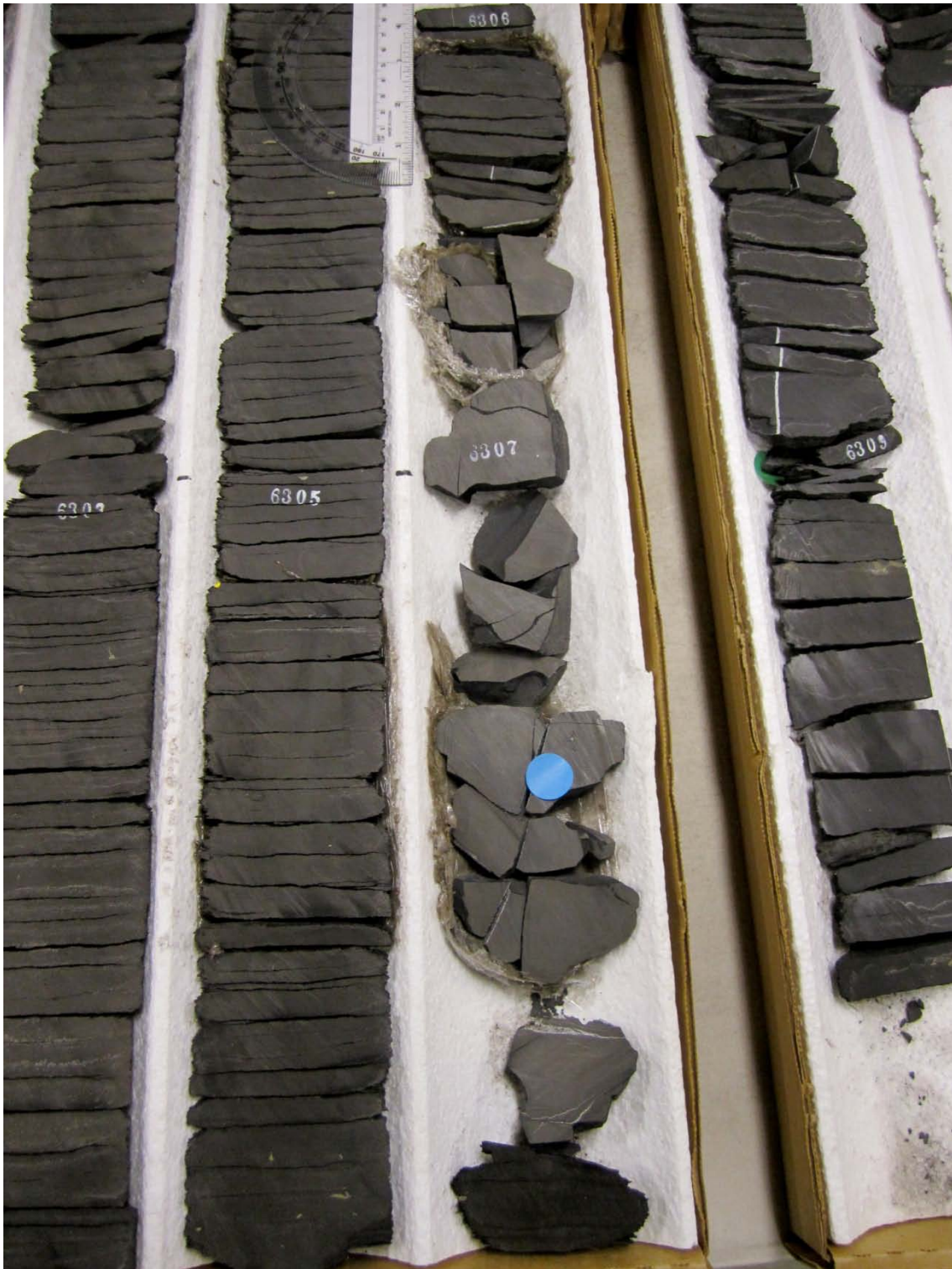
Figure 20. Bottom box of Stewart Nancy unit #4 core showing 'poker chip' breaks in the mudrock interval. A fracture network sealed with calcite and pyrite occurs in the paler grey carbonate concretion and vertical, calcite-sealed fractures are present at the base (6,302 to 6,310 ft).
