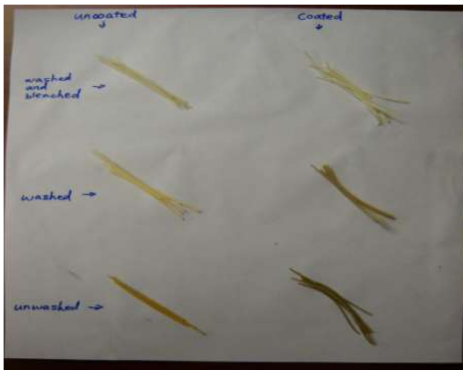
Figure 18: Coated and non-coated fibers treated with different cleaning reagents. Left: uncoated fiber, from bottom up: untreated, washed with acid /base, washed with acid/base and bleached; Right: coated fiber, from bottom up: untreated, washed with acid/base, washed with acid/base and bleached.
