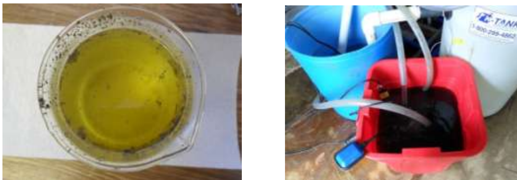
Figure 14: Oil residue/particulates collected during citric acid cleaning (left), and a dark solution collected during caustic cleaning (right) representing predominantly organic foulants adhering to the membrane.
