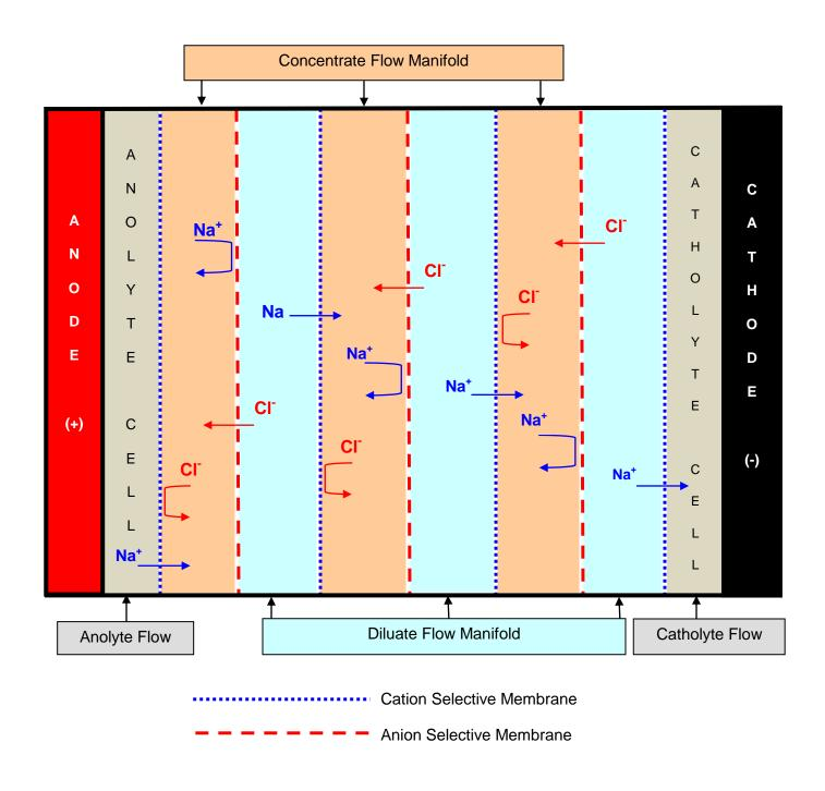
Figure 2: Ion Flow in an Electrodialysis Stack
