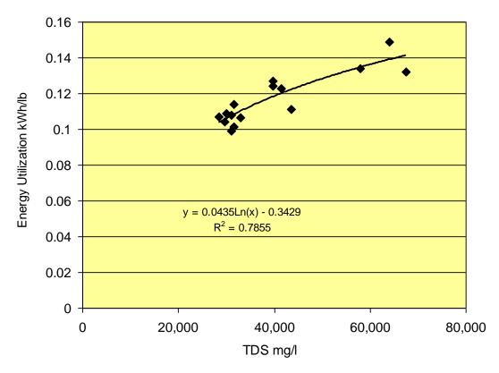
Figure 19: Energy Efficiency vs. Initial TDS
