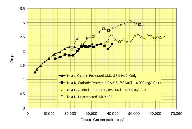
Figure 23: Protection of Electrolyte from Calcium Incursion with Single CXM-S Membrane at the Cathode Boundary
