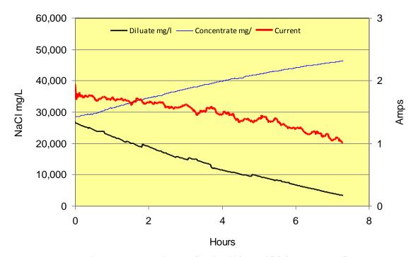
Figure 7: Test B; 3% NaCl with 30/gl Na2SO4 Electrolyte 5V
