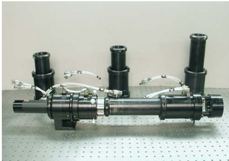
Figure 84. Collimator for HPFL collimates beam from 0.25" to 1"
