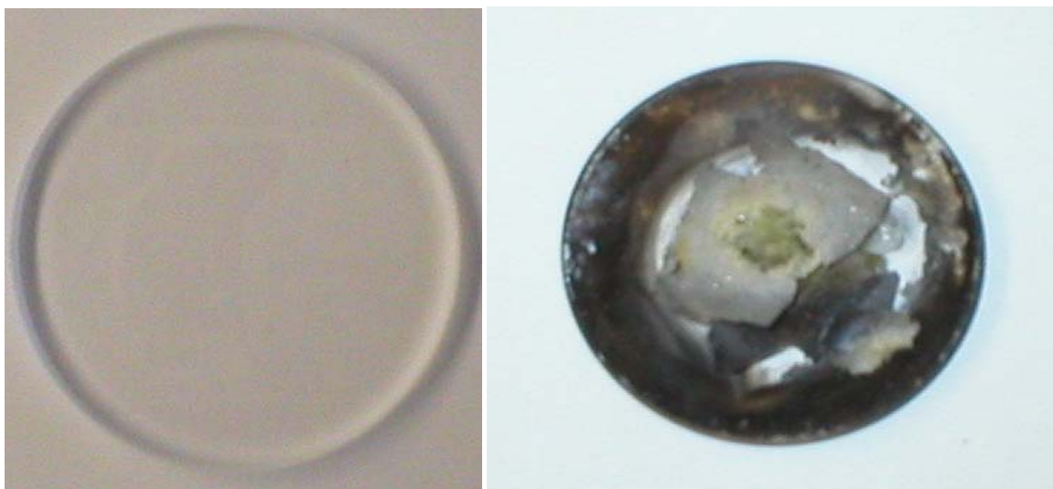
Figure 91. High pressure perforation cell cover lenses before and after lasing for prove of concept experiment.
