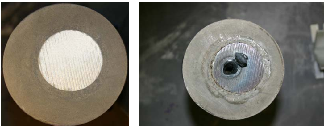
Figure 28. Pre- and post-lased images of 10.16 cm (4.0 in) diameter by 15.24 cm (6.0 in) length limestone core inset with 5.08 cm (2.0 in) diameter by 1.27 cm (0.5 in) thick steel plate.
