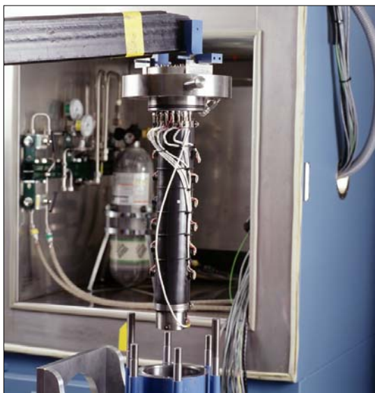
Figure 7. Instrumented sleeve held above reaction cell.
