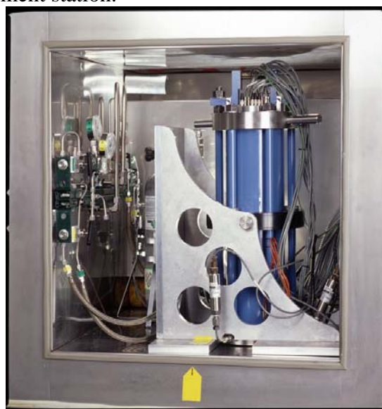
Figure 8. Assembled reaction cell inside temperature controlled chamber.
