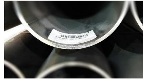
In the Pipeline Industry - Material Traceability is the ability to trace all materials used to construct a piping system back to their origins.
