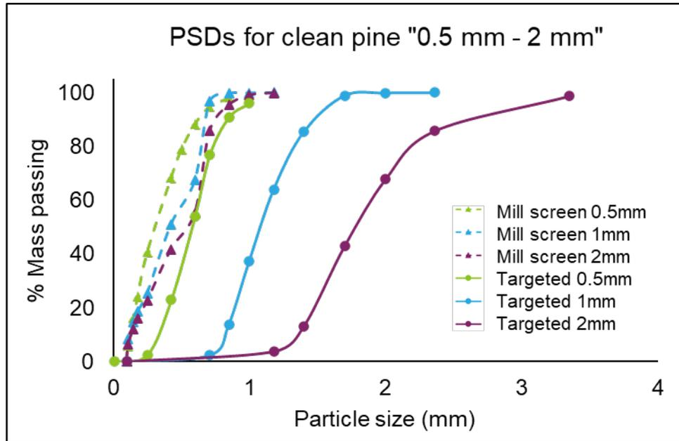
PSDs developed based on mill screen size and targeted particle mean size
