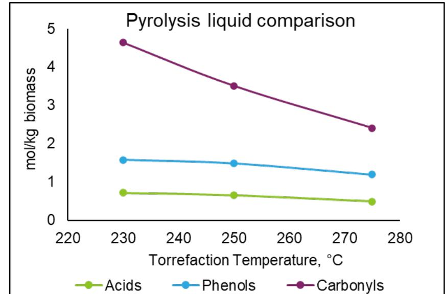
Quality of pyrolysis oil improves with torrefaction due to decreasing water, carbonyls and acids
