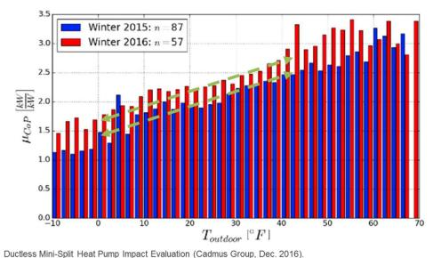
Cold ambient temperatures lower heat pump efficiency (COP) by 30-50% (or more).
