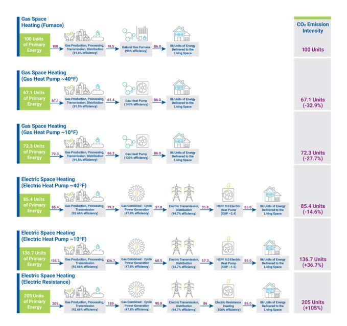
Figure 14: Full-Fuel-Cycle Comparisons of Gas and Electric Heating Pathways
