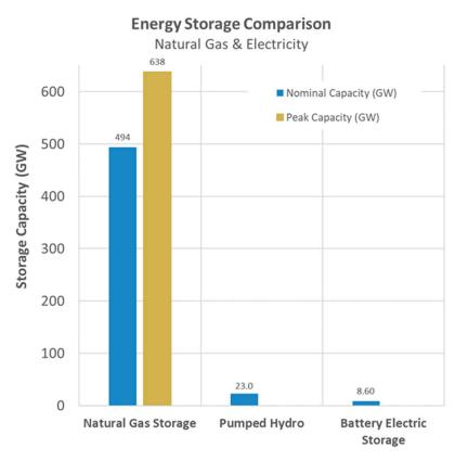
Figure 49: Nominal Energy Storage Capacity (DOE-EIA)
