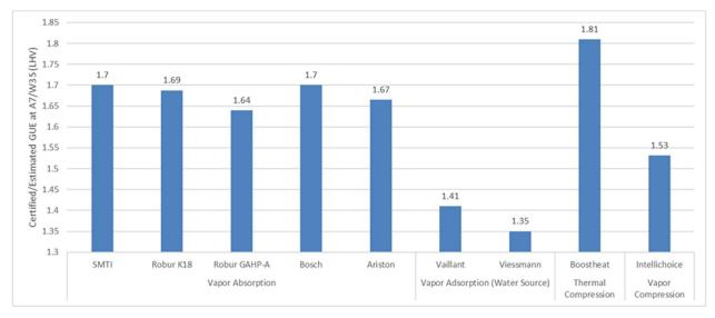
Figure 20: Example Natural Gas Heat Pumps and Efficiency
