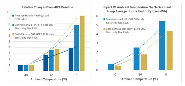
Figure 12: Impact of Ambient Temperature on Electric Heat Pump Electricity Use
