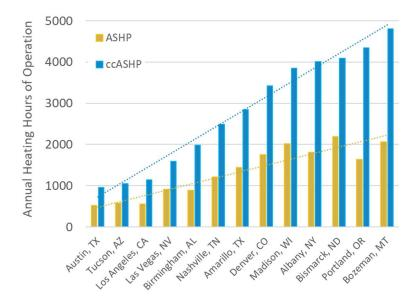
Figure 13: Electric Heat Pump Annual Heating Operating Hours in Different Climates (Source: GTI Energy)
