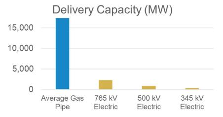
Figure 48: Major Natural Gas and Electric Transmission System Capacity (DOE, AEP)
