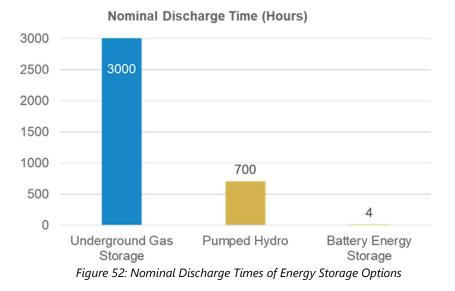
**Main Finding**: Electric energy storage options have higher cycle losses than natural gas systems and battery energy storage systems lack the seasonal capability needed to meet winter electricity loads resulting from large-scale residential electrification. Pumped hydro storage has seasonal capabilities but has not had new investment in recent years.
