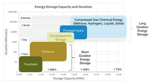
Figure 51: Size and Duration of Energy Storage Systems (adapted from National Hydropower Association report)
