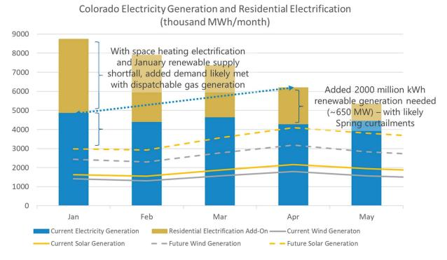
Figure 34: Combined Challenges of Electric Space Heating and the Shortfall of January Renewable Generation Supply (DOE-EIA, GTI Energy)
