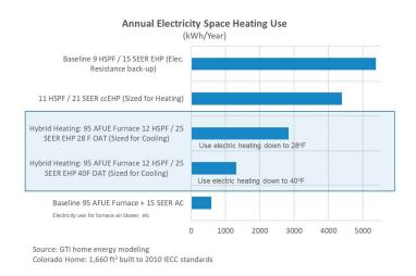
Hybrid natural gas and electric heating systems – a high-efficiency gas furnace with an electric heat pump operating at milder winter temperatures – results in lower peak electricity use.
