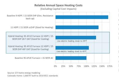
Hybrid natural gas and electric heating systems – a highefficiency gas furnace with an electric heat pump operating at milder winter temperatures – results in lower consumer cost impacts.
