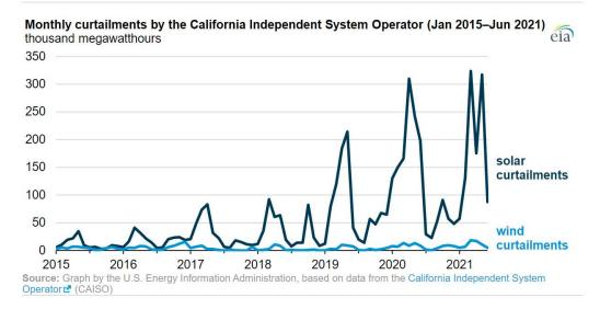
Figure 32: California ISO Solar and Wind Curtailments (DOE-EIA)
