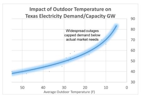
Figure 17: Impact of Cold Temperatures on February 2021 Texas Electricity Demand
