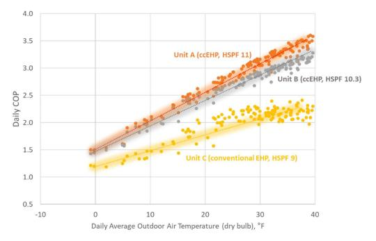
Figure 11: Electric Heat Pump Performance Below 40°F (Source: GTI Energy)
