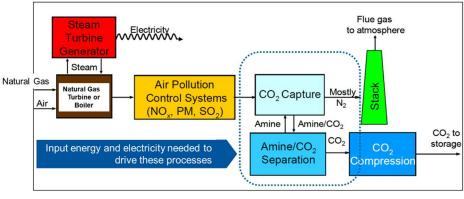
Adapted from: **Source:** E. S. Rubin, "CO<sub>2</sub> Capture and Transport," *Elements*, vol. 4 (2008), pp. 311-317. *Figure 39: Example CO<sub>2</sub> Capture Process*
