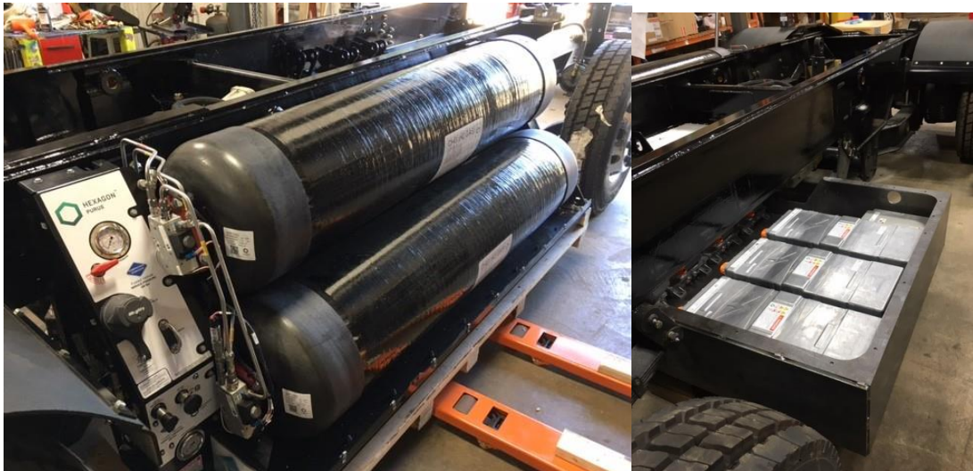
Figure 7 - Vehicle energy storage systems (H2 tanks and Batteries) installed onto rolling chassis
