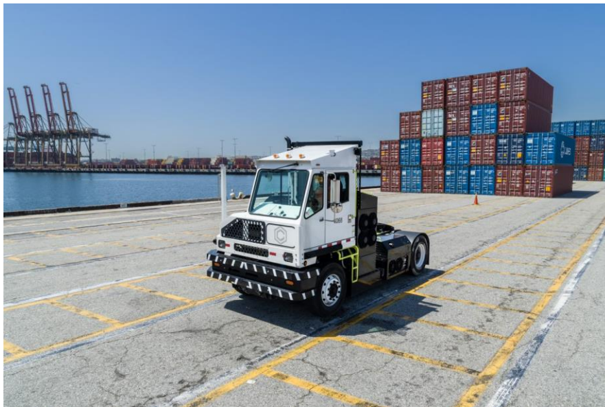
Figure 32 - Capacity Trucks terminal tractor at Port of Los Angeles
