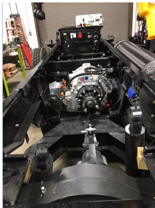
Figure 8 - Rear view showing Traction Motor during vehicle build
