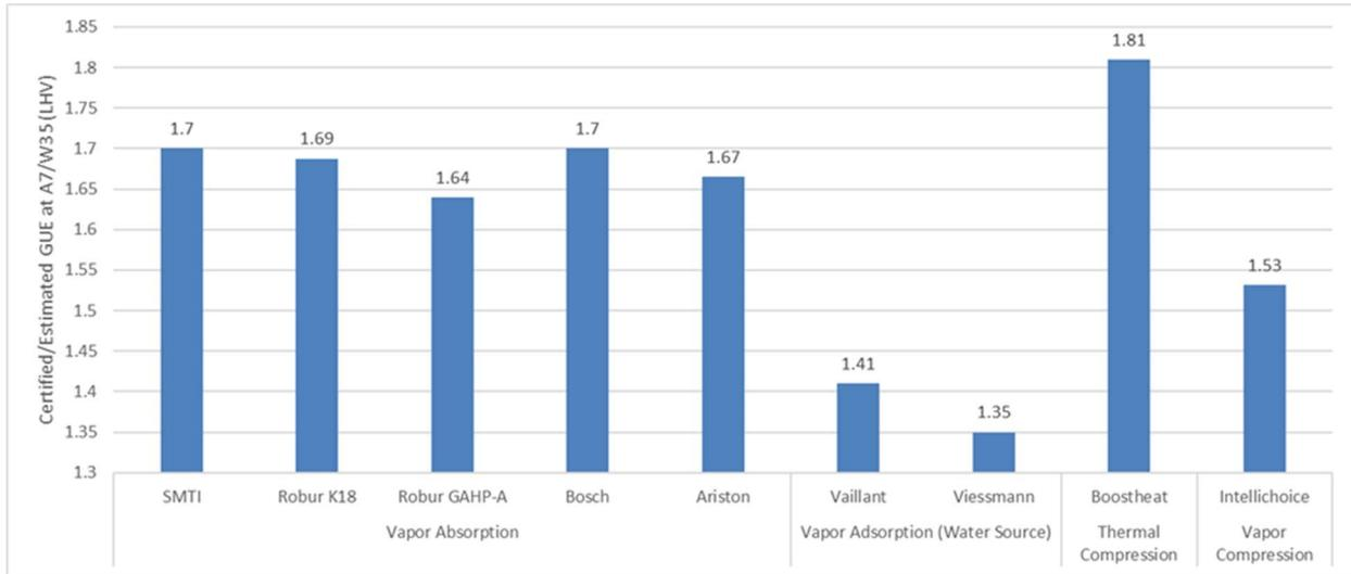
Figure 20: Example Natural Gas Heat Pumps and Efficiency
