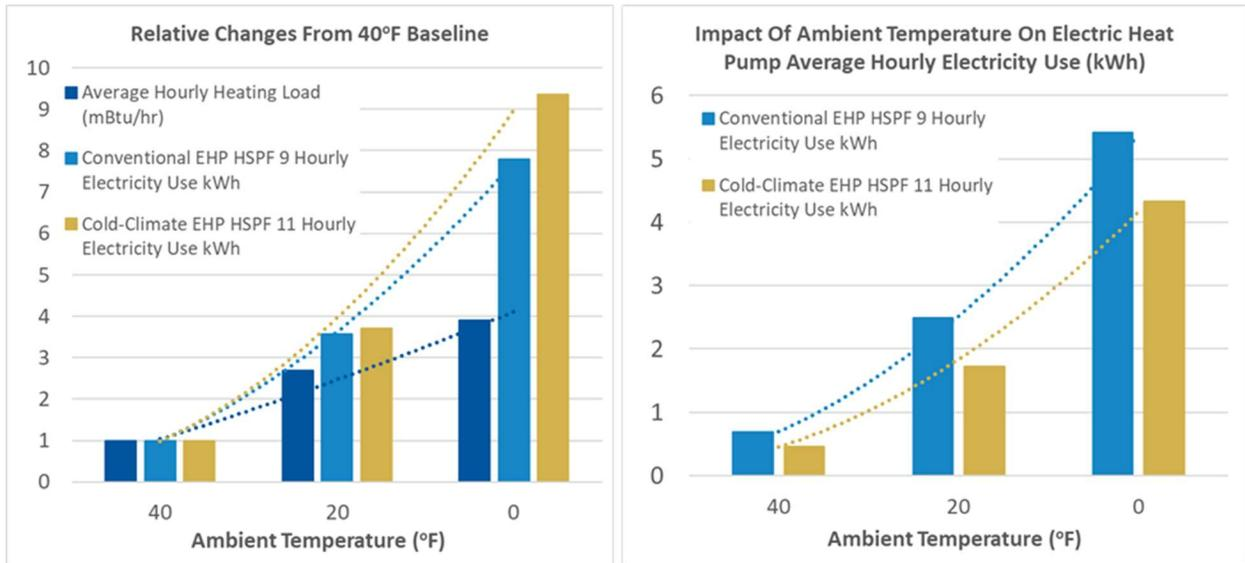
Figure 12: Impact of Ambient Temperature on Electric Heat Pump Electricity Use
