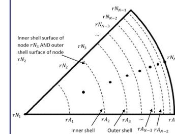
The particle interior model is based on Whitaker's Finite Volume Model<sup>1</sup>. One or more spherical particles are formed as feedstock. The conservation of energy, conservation of mass of water, and conservation of mass of air in conjunction with material properties such as diffusivity and true particle density are utilized to determine mass and energy migration within each particle.
