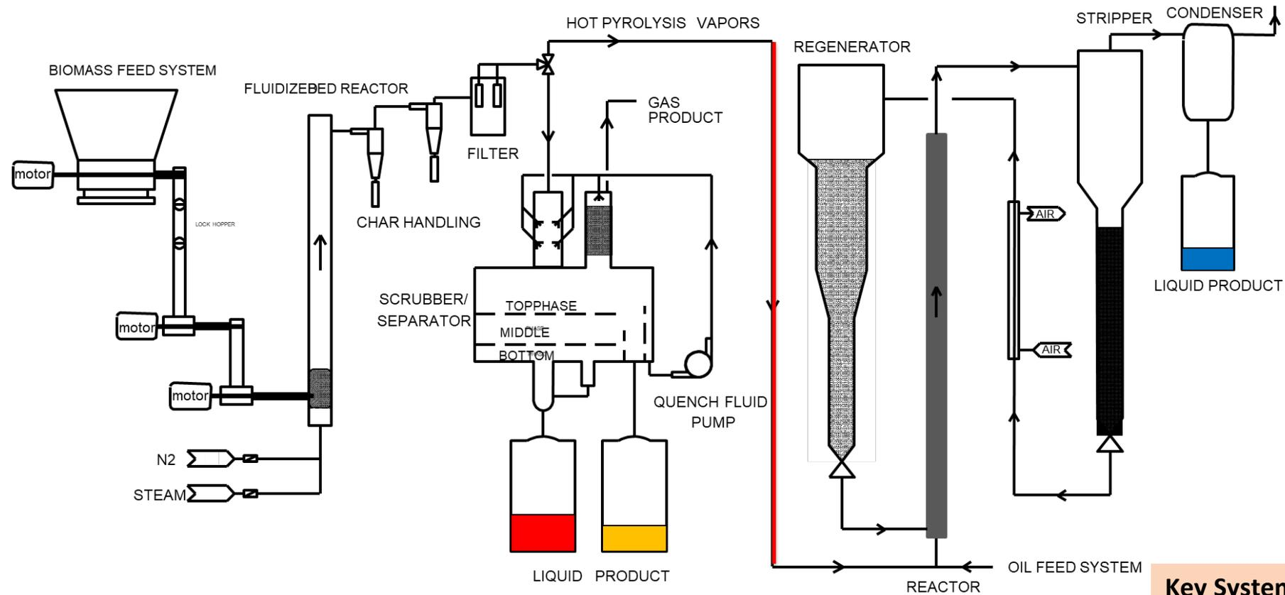
The Davison Circulating Riser System when coupled with a biomass pyrolyzer is used to generate bio-oils from a riser reactor leveraging zeolite-based catalysts
