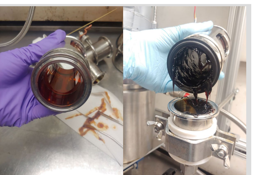
Pyrolysis products collected in ESP (left – stem wood, right – R:B:N 1:2:2)
