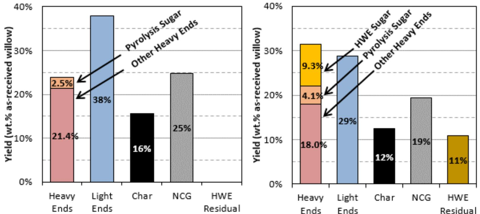
Yields from autothermal (air-blown) pyrolysis at 500 °C of (left) as-received willow; (right) HEC willow. Product yields of HEC willow are normalized to as-received willow and include sugar and residual yields from extraction process. Total yield is greater than 100% due the reaction of oxygen with products.
