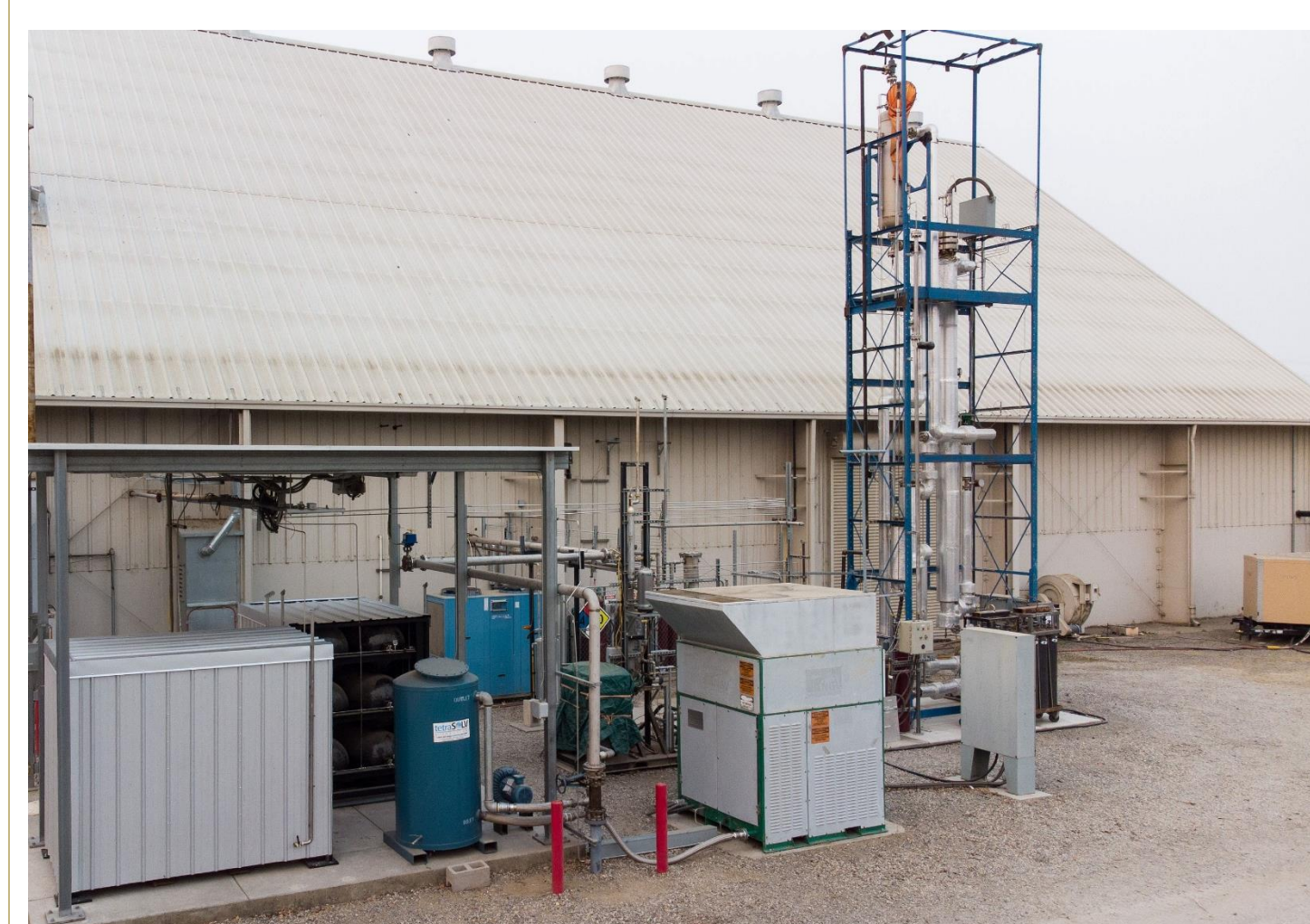
Fig. 3: Bench-scale MAS system at West Biofuels
