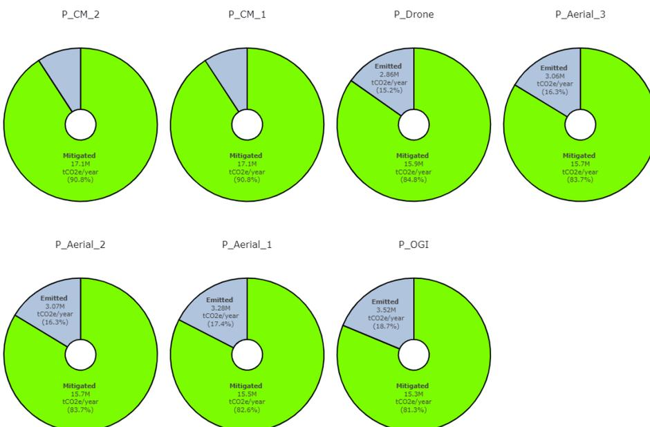
**Figure 16: Breakdown of emissions (CH<sub>4</sub>) by program (emitted = slate, mitigated = green) at Barnett compressor stations over 5 years with 4x annual OGI surveys / 6x screenings with OGI FU and 1x OGI annual survey.**
