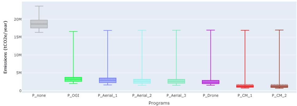
**Figure 18: Breakdown of mitigated emissions by initial detecting program at Barnett compressor stations.**
