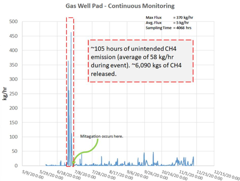
**Figure 10. Example of an emission detection leading mitigation with a CM system.**
