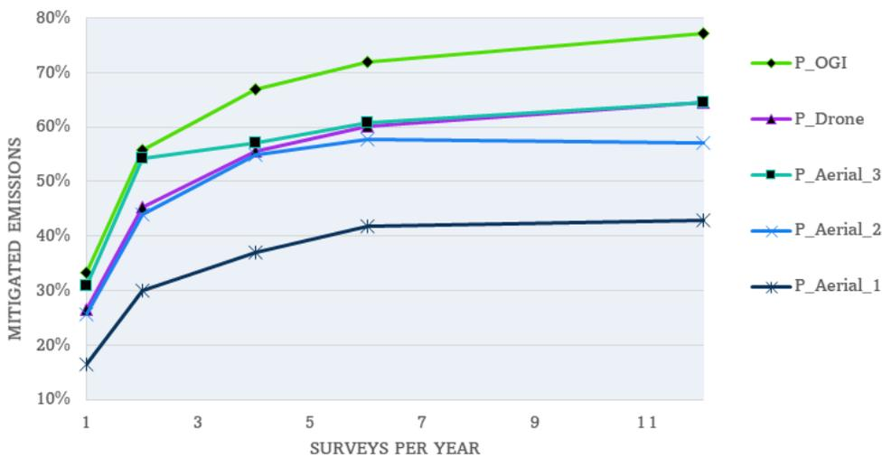
Figure 24: Estimated emissions mitigation from the use of different technologies on production sites in the Barnett with different survey frequencies.
