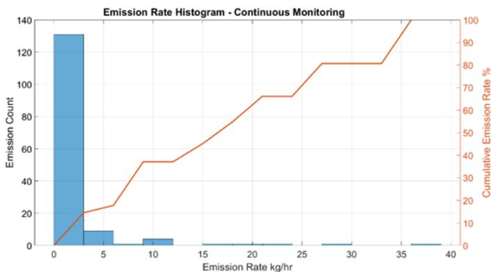
**Figure 5. Emission rate histogram for a 91-hour period for a CM monitor at a single site**
