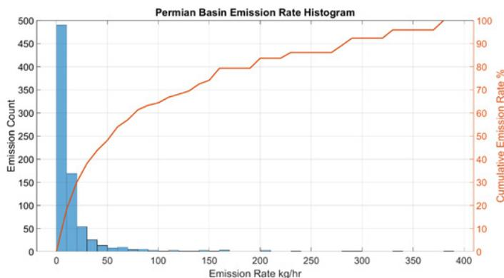
**Figure 3. Histogram of all emission sources provided using low-altitude aerial remote sensing technology.**
