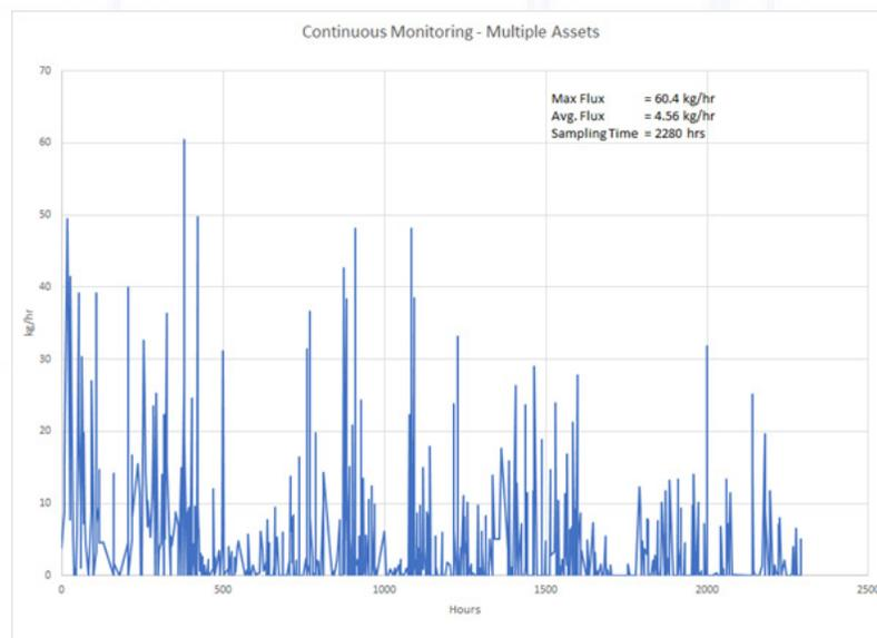
**Figure 9. Time series of 2,200 hours of data from a CM sensor in Permian Basin.**
