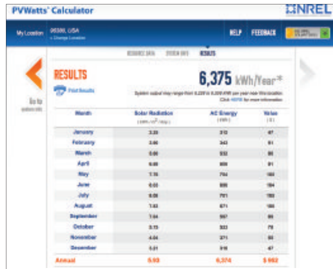
Fig. 3.2 Estimate solar production early, to establish roof orientation Web-based calculator - National Renewable Energy Laboratory.
