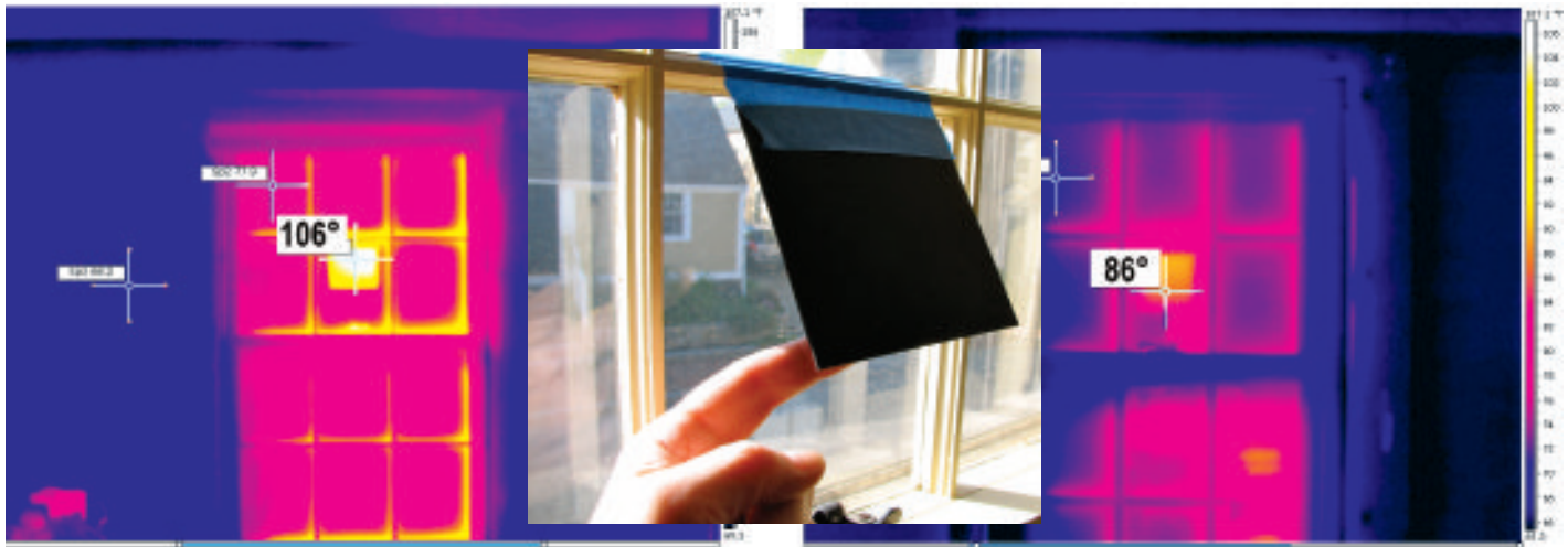
Fig. 3.4 Low SHGC keeps solar heat out of the house
