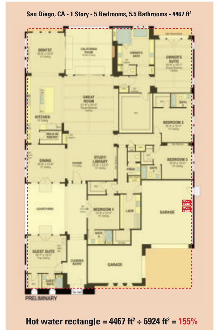
Fig. 8.5 Water heater in the garage? Bad idea.
