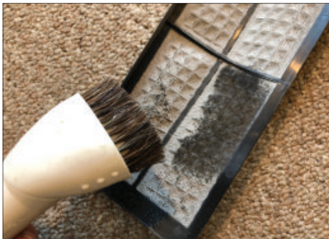
Fig. 10.4 Most exhaust air filters are easily cleaned with a vacuum
