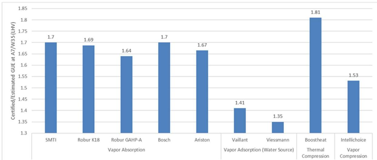
**Figure 11: Example Natural Gas Heat Pumps and Efficiency**
