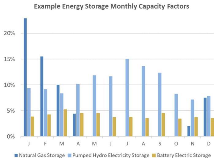
**Figure 42: Example Energy Storage System Capacity Factors (DOE-EIA)**
