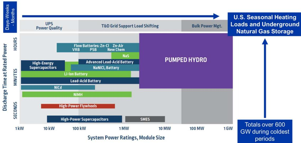
**Figure 43: Size and Duration of Energy Storage Systems**
