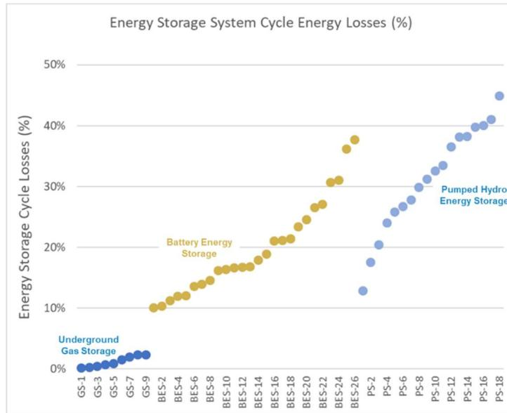
**Figure 41: Energy Storage Cycle Energy Losses (DOE-EIA, GTI)**
