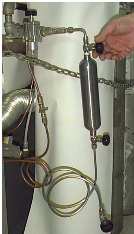
**Note:** Any sampling lines or control devices should be constructed from materials that are inert and non-sorbing. Type 316 stainless steel is preferred. Non-permeable and non-reactive plastic tubing may be used for low pressure gas sampling. All cylinders supplied by GTI for sampling are evacuated to a hard vacuum, and shipped with closed valves and plugged outlets.
