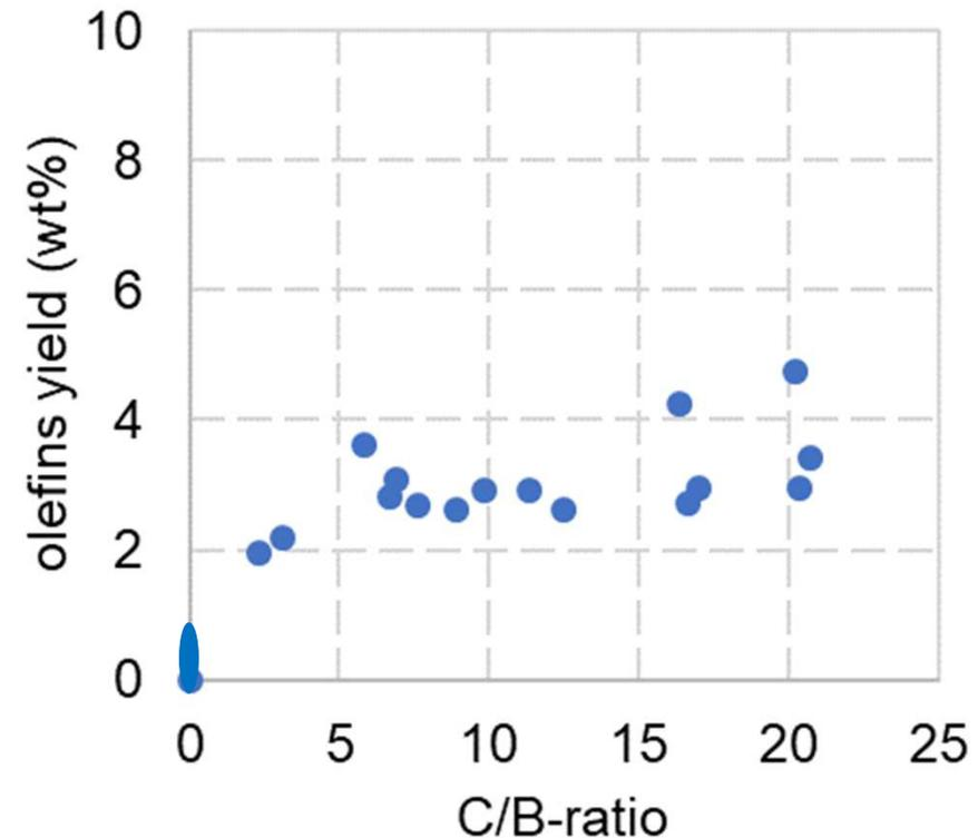
No catalyst → negligible BTX and olefins (ethylene+propylene)
