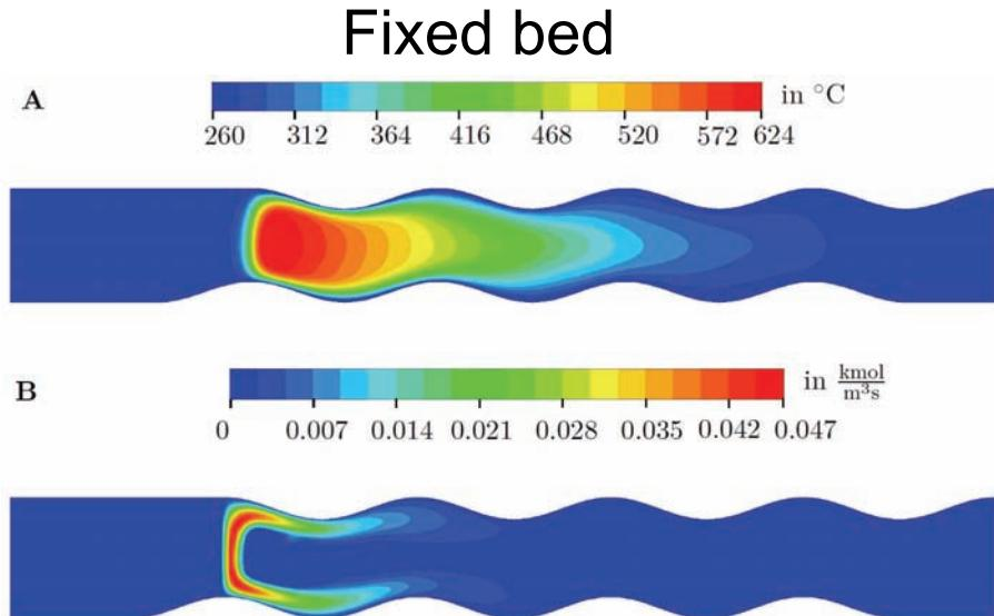
CFD model is capable of predicting temperatures for a broad variety of geometries and conditions
