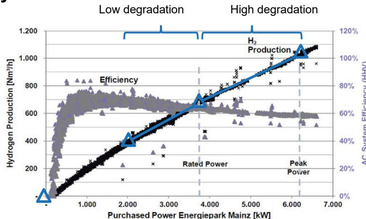
Piece by piece interpolation of the characteristic curves for load-dependent H<sub>2</sub>-production and efficiency
