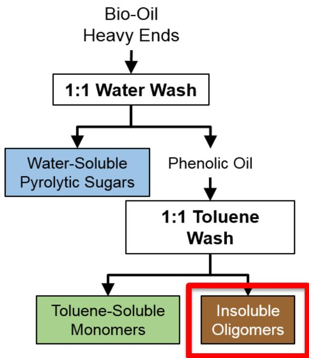
Liquid-Liquid Extractions of Bio-Oil Heavy Ends
