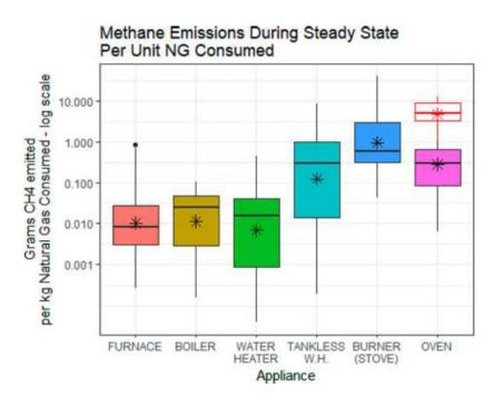
From this testing, most methane emissions stem from equipment start-up and shut down. In fact, at steady-state operation M&F find instances where furnace methane emission levels are lower than background ambient methane concentration (i.e., furnaces in some instances consume ambient methane during steady-state operation). Even factoring in on/off cycles, this study finds very low methane emissions from gas furnaces.
