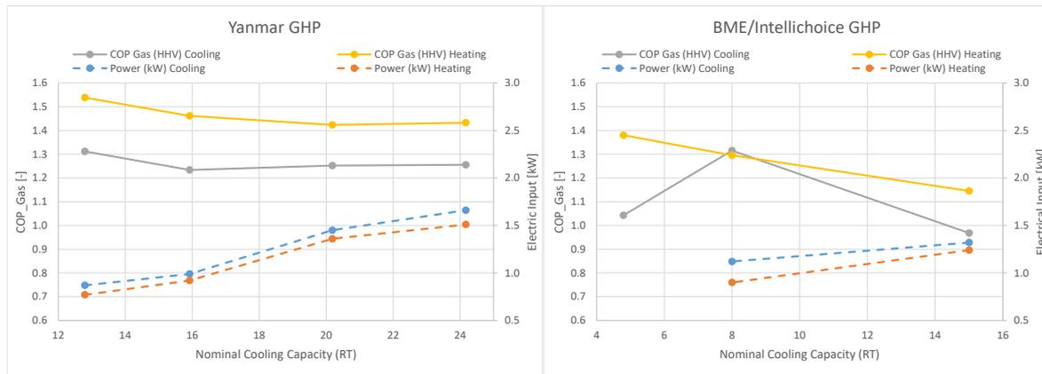
Figure 3: GHP Efficiencies and Power Consumption [Yanmar & BME, 2018]
