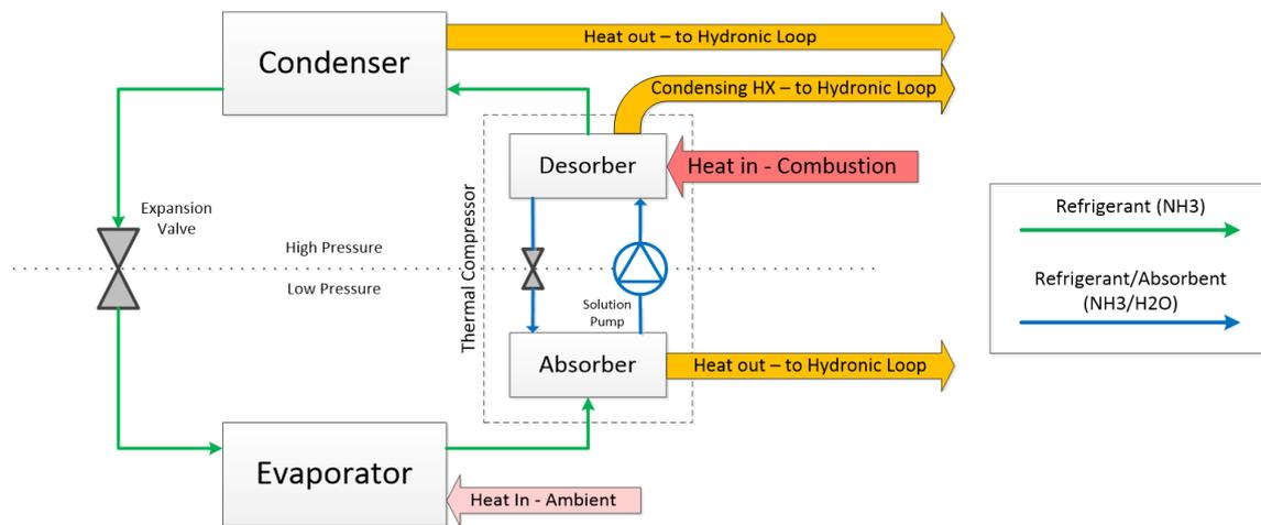
**Figure 2: Simplified Diagram of Single-Effect Absorption Cycle**
