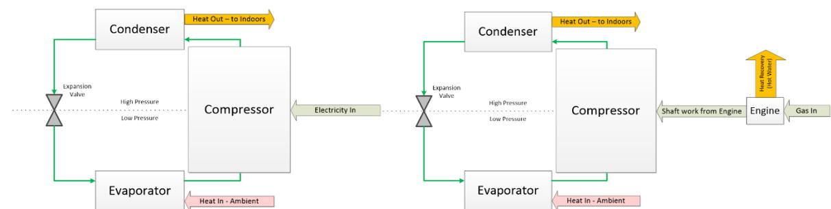
**Figure 1: Simplified Diagrams of an Electric-Driven (left) vs. Gas-fired Engine-Driven Vapor Compression Cycle (right) – Heating Mode**
