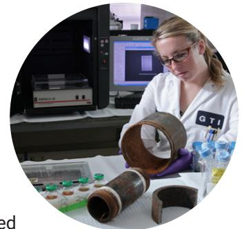
Quantitative polymerase chain reaction (qPCR) measures specific genes essential for the metabolism of corrosion causing bacteria in the samples. The method is far more
