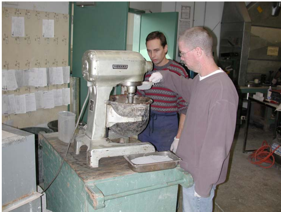
Photograph 2 – Utilibond bonding compound being prepared for testing.
