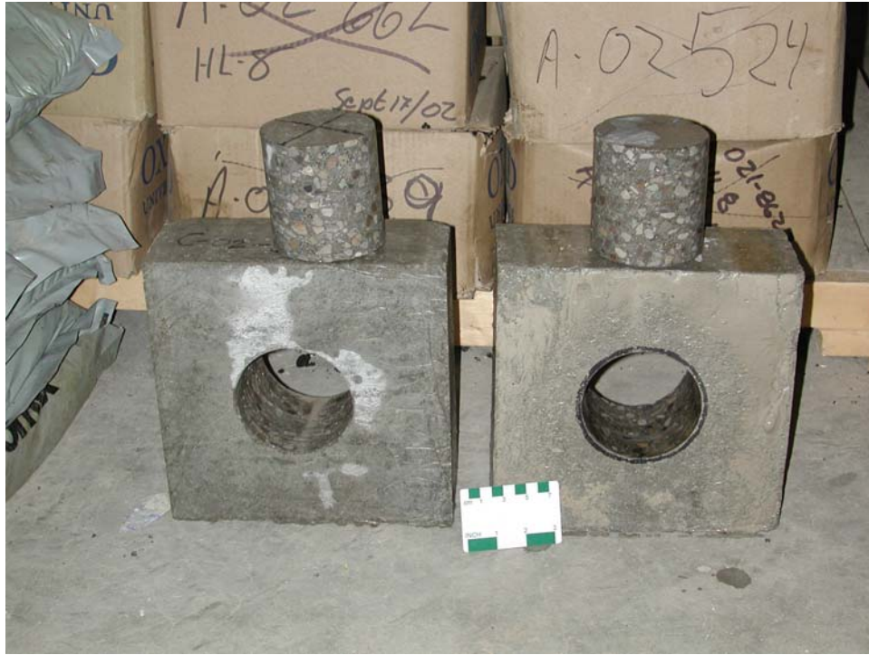
Photograph 1 – Test slabs with samples removed.
