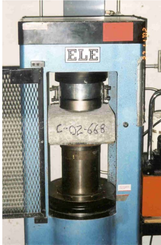
Photograph 5 – Testing configuration in compressive strength machine.
