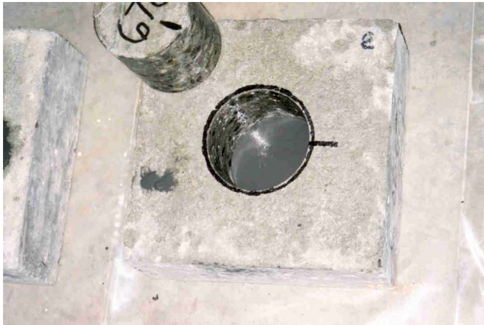
Photograph 3 – Core sample being placed into test panel.
