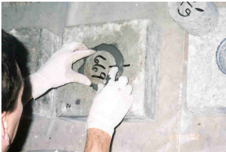
Photograph 4 – Core sample being placed into test panel.
