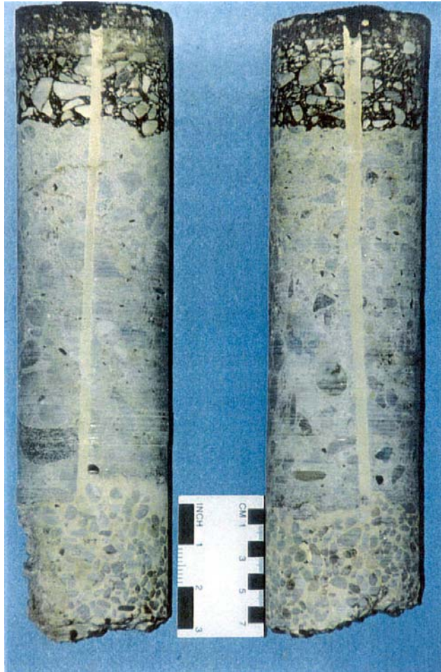
Photo 5 – View of satellite cores taken one month after installation in 1995.
