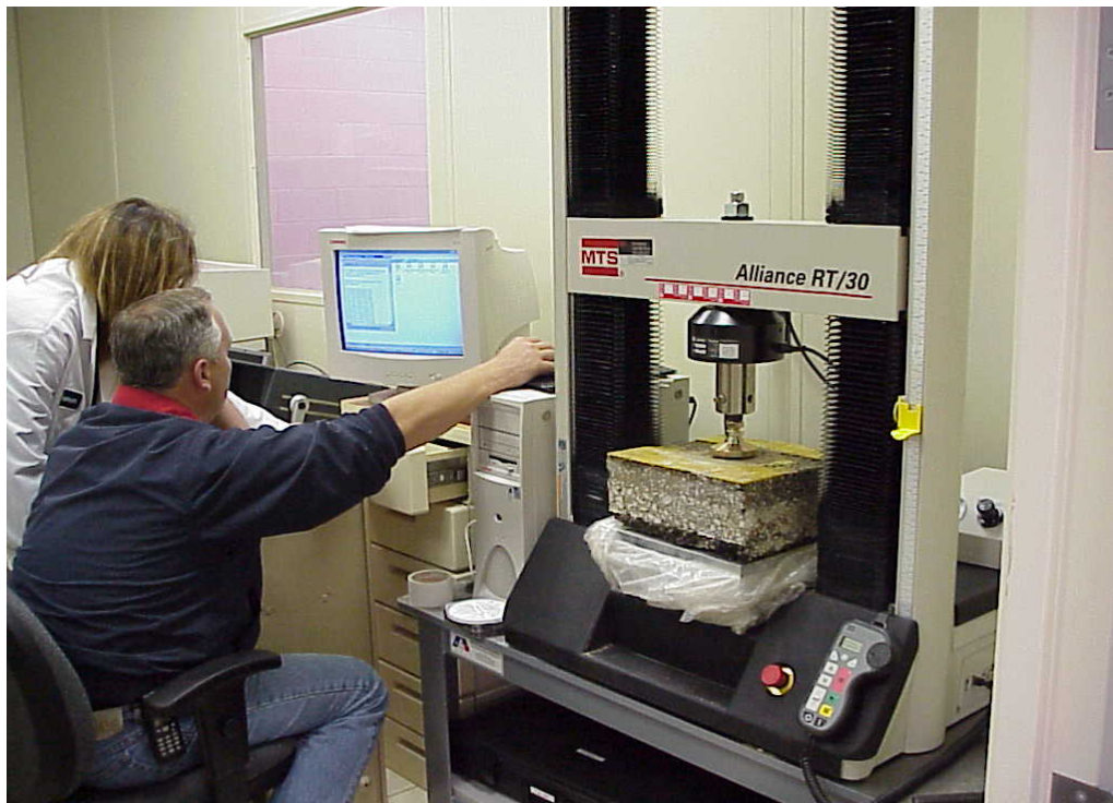
Figure 4. Lab test to evaluate the 30 & 60-minute shear strength of the grout
