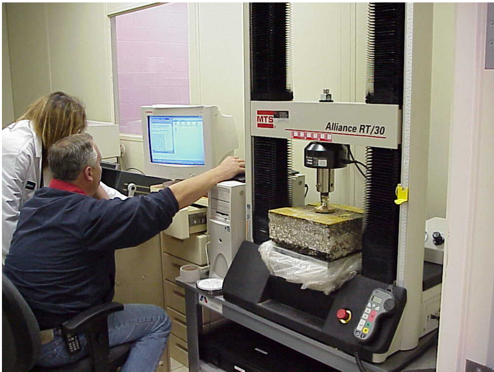
Figure 4. Lab test to evaluate the one-hour shear strength of the grout
