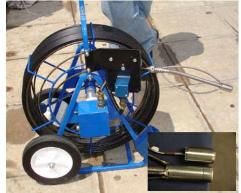
Above: Keyhole camera and reel Inset: Keyhole camera vs. conventional camera
