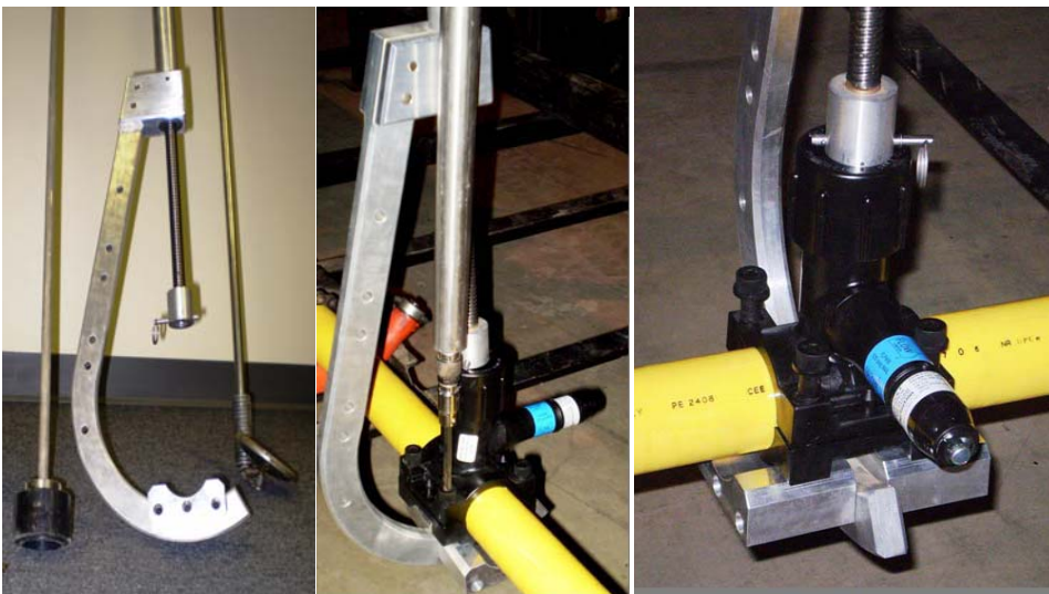
Omega's tools include standard extension handles that engage pneumatic heads; quick-release handles for pickup and placement manipulations; and torque handles to generate torque force. Numerous attachments in the form of specialized sockets and manipulation devices are used to accomplish specific tasks.
