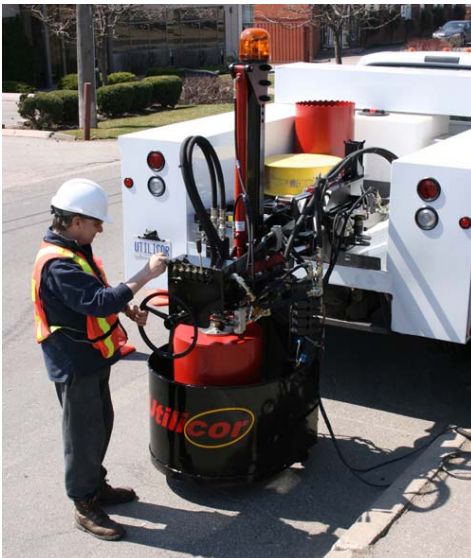
The unique Traversacor ™ system allows for coring up to 28 inches out from the back of the truck and from the curb to more than halfway across the width of the truck, without repositioning the vehicle.
