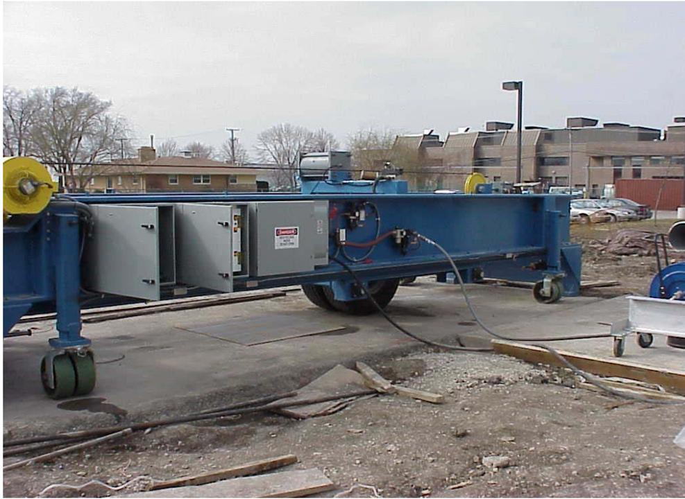
Figure 42. View of the Accelerated Pavement Loading Equipment
