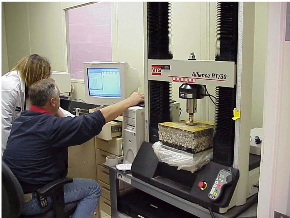
Figure 6. Performing the shear test using the MTS testing machine
