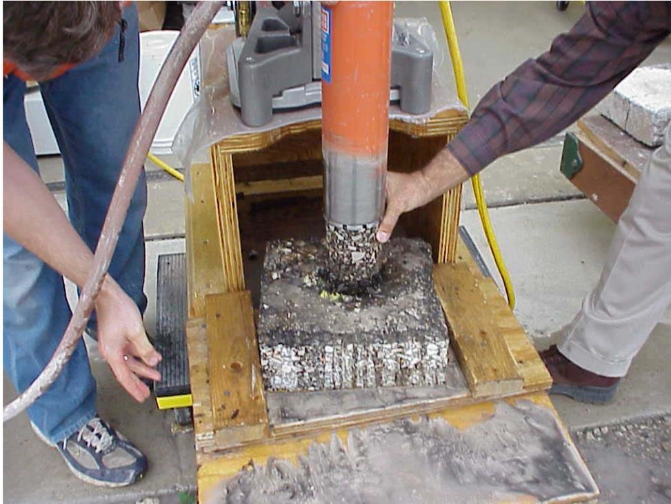
Figure 3. Retrieving the core sample from the drilling machine
