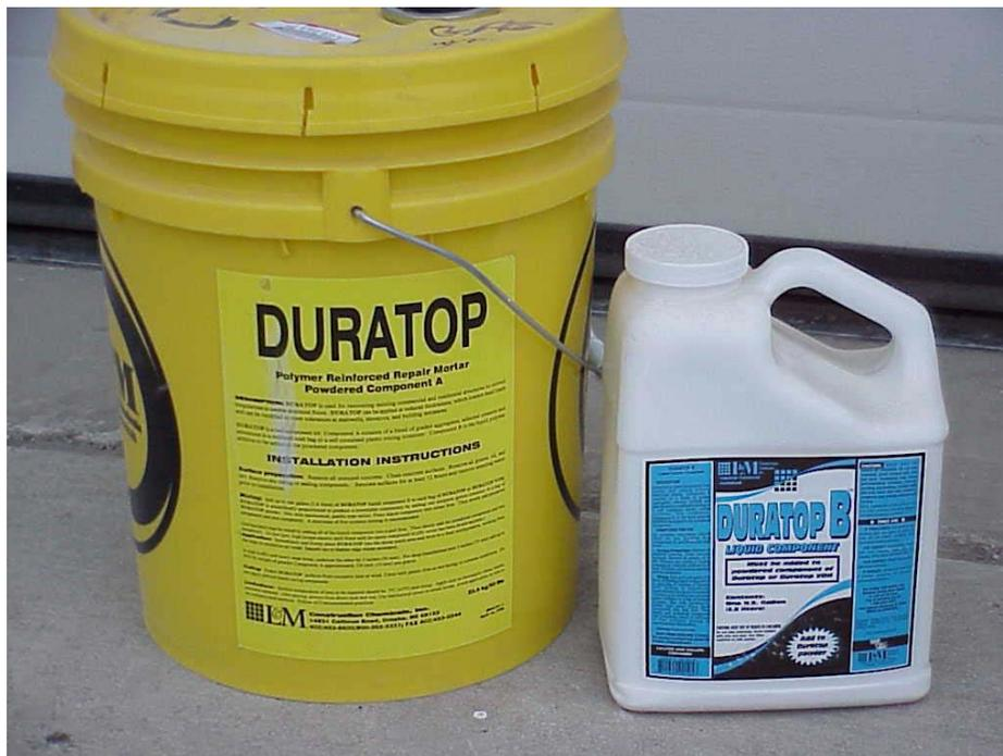
Figure 9. The two components mix of the Duratop grout
