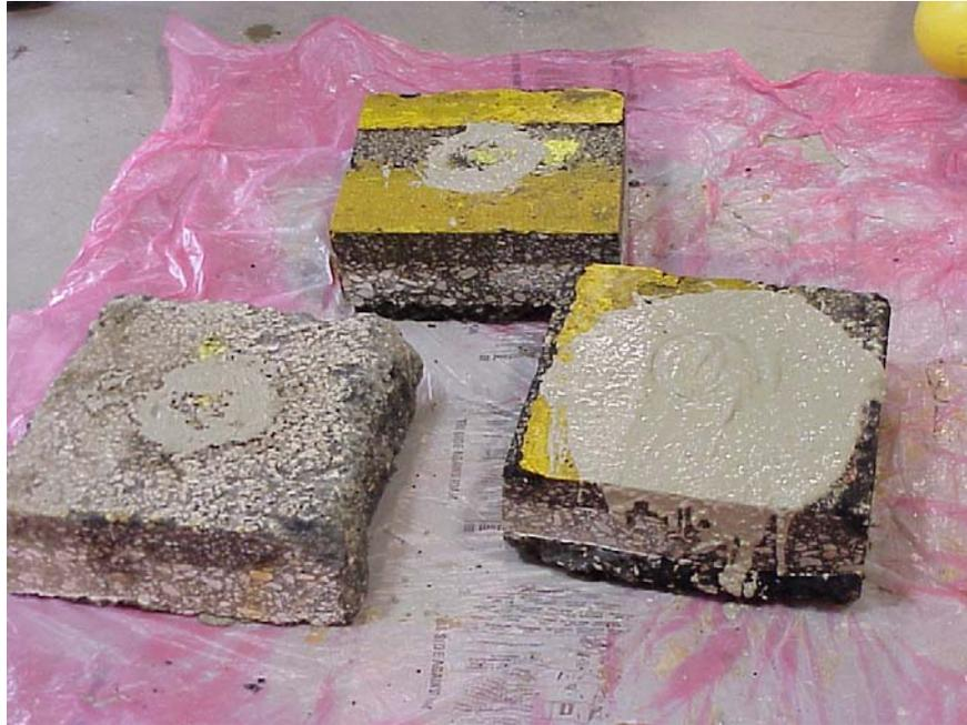
Figure 4. View of several samples prepared with various water content ratios
