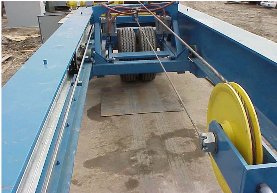
Figure 43. Front view of the APLE showing the dual tire loading on the core section
