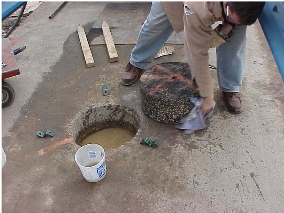
Figure 39. Cleaning the surface of the cores.
