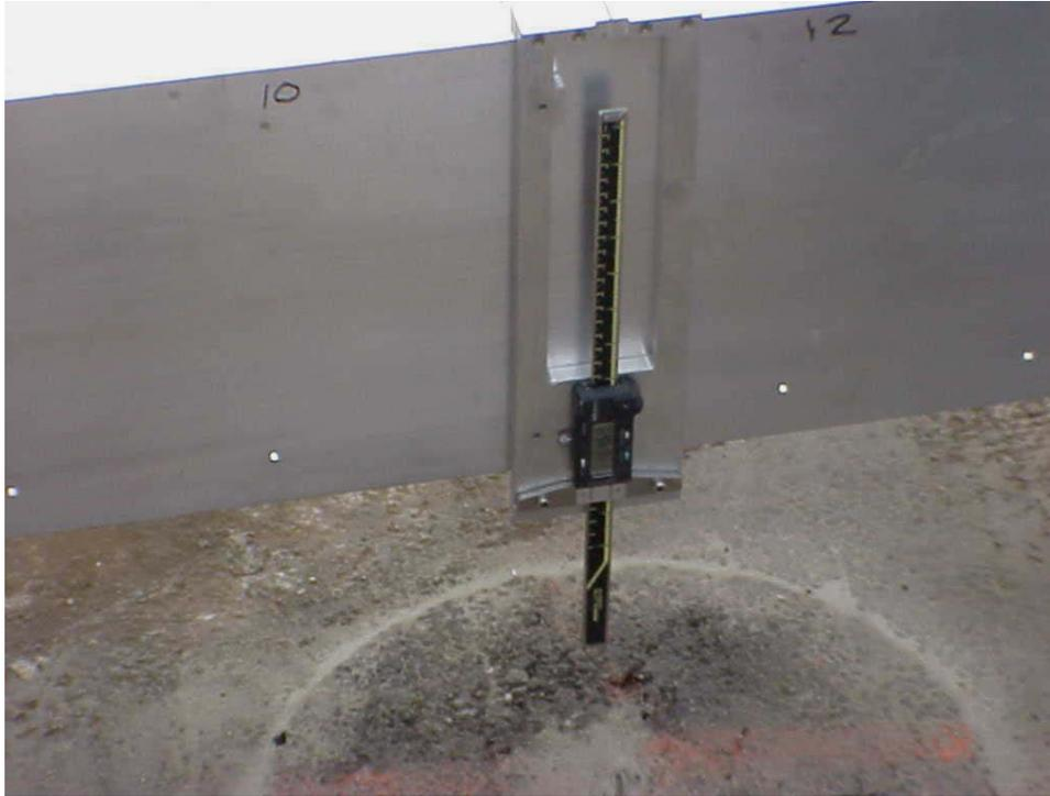
Figure 47. View of depth measurement using the depth gauge
