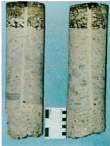
Figure 6. Satellite core samples taken through bonded area of reinstated core show effective coupling.
