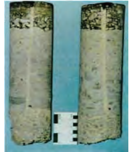
Satellite core samples taken through bonded area of reinstated core. The light gray line is Utilibond showing excellent bonding of asphalt-concrete core (central area) and undisturbed pavement (outer layer).
