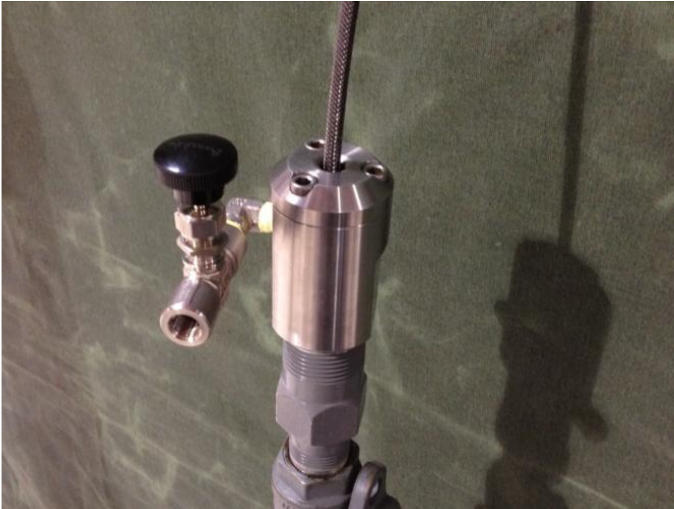
Jameson Stuffing Box used for Mini Duct Hunter can be used to launch camera through service riser stopcock
