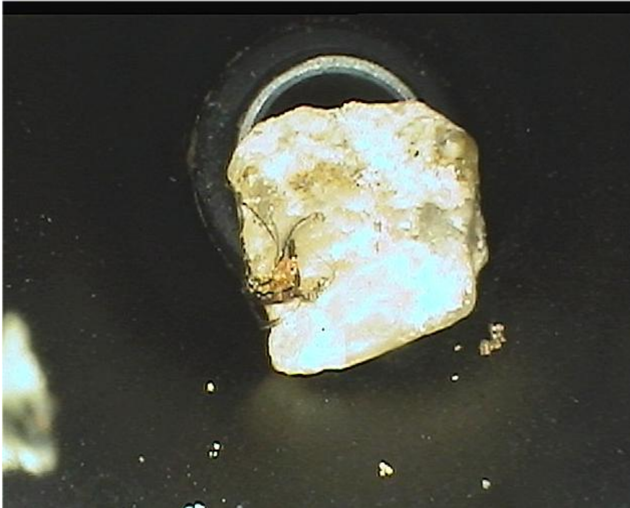
Small pebble restricting flow on 1/2" PE service in Yuma Arizona
