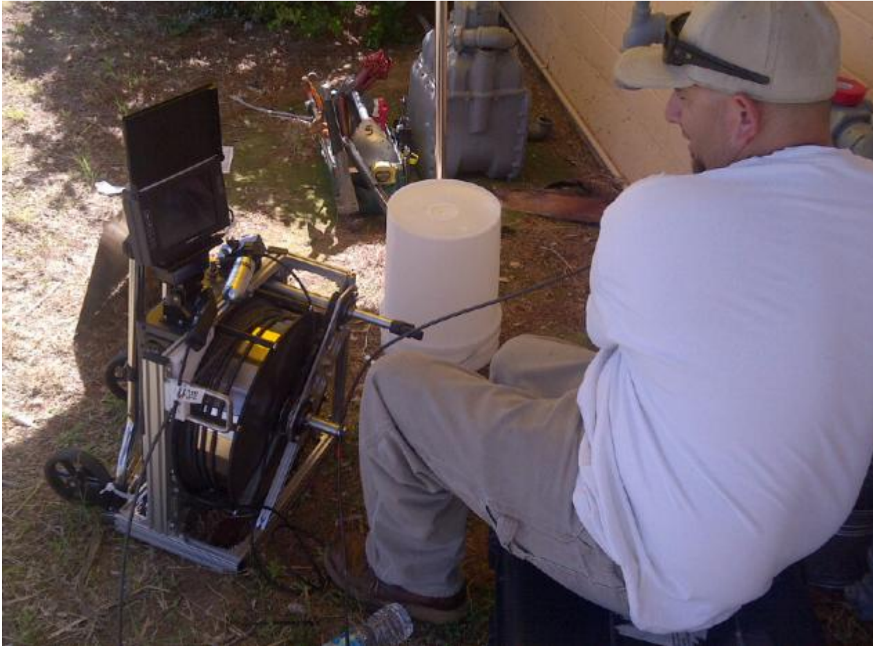
8 mm camera being tested for 1" pipe size only
