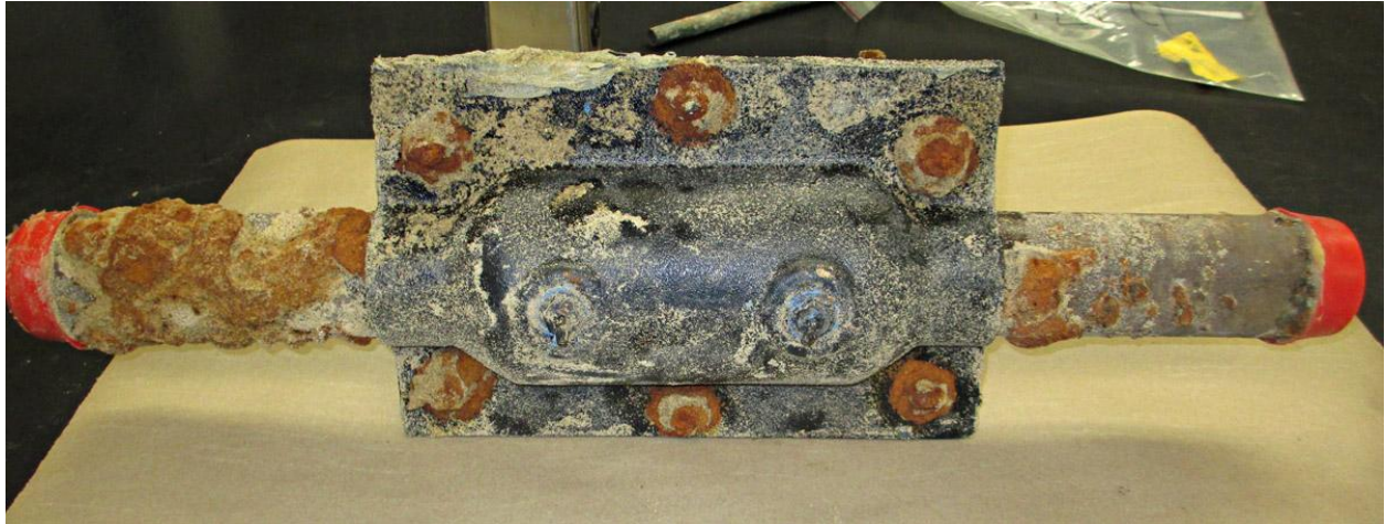
Figure 6 Test specimen after removal from corrosion chamber
