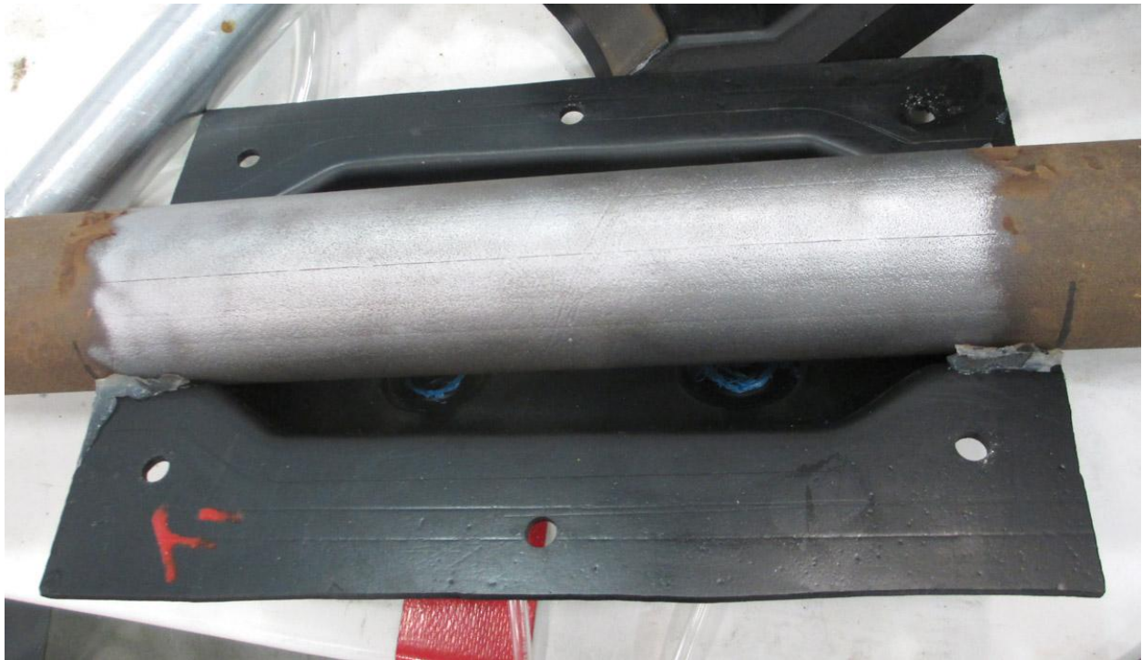
Figure 1 Surface of 2" pipe after grit blasting
