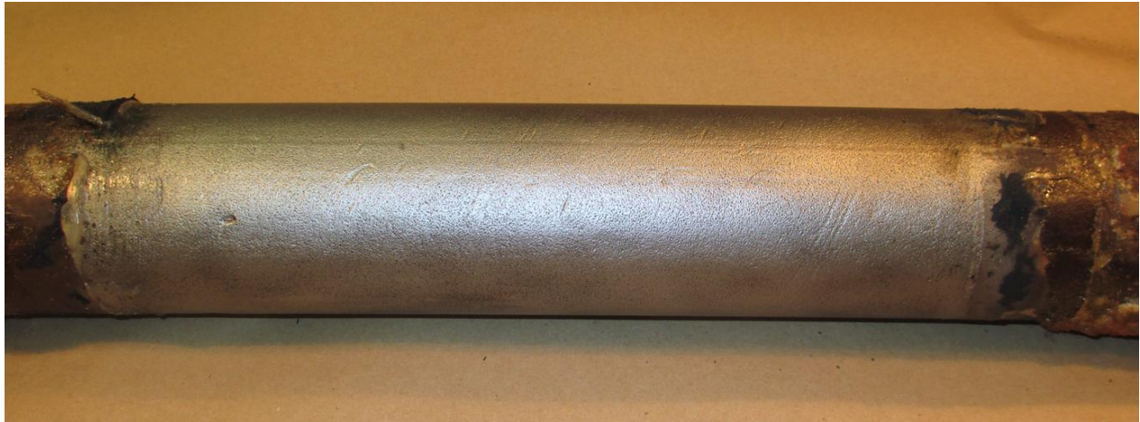
Figure 8 Test specimen after removal of all residual wax
