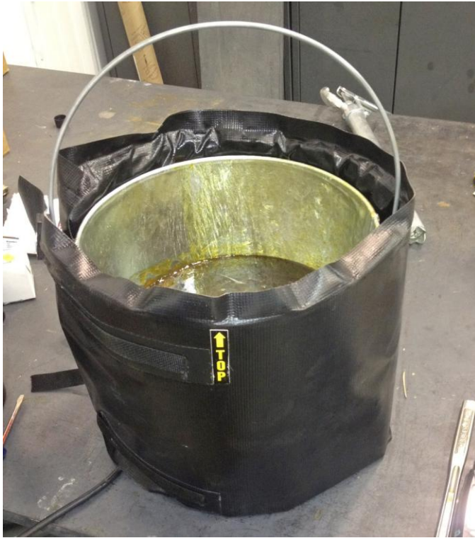
Figure 2 Liquefied Trenton wax-tape primer after heating with bucket warmer
