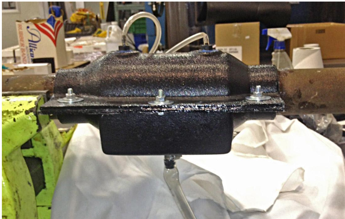
Figure 3 Enclosure before filling
