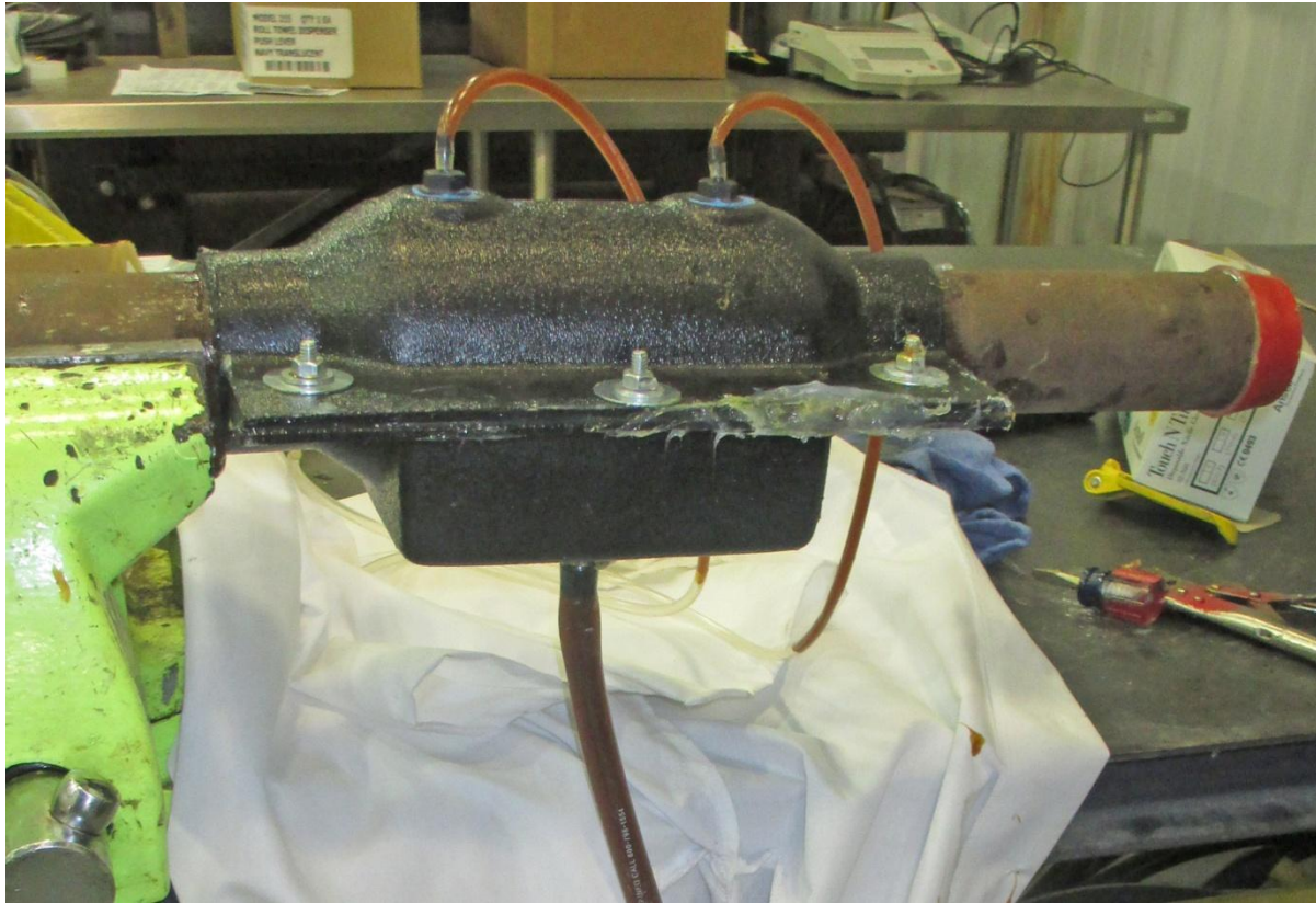
Figure 4 Enclosure after filling with melted wax
