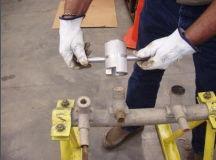
Flip the scraper/peeler with side “B” facing down (flat side of scraper) - scrape outside diameter of tee stack again.
