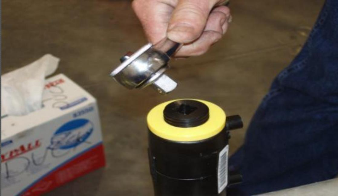
Use a standard  $\frac{1}{2}$  " square drive to turn the plug into the Insert. The top of the Plug should be flush with the top of the Insert.
