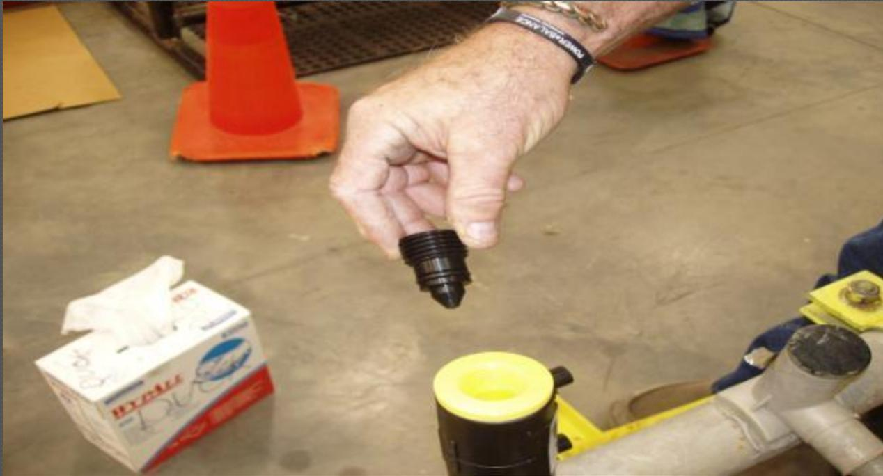
Install the Plug Repair Fitting with the lubricated o-ring into the Insert.
