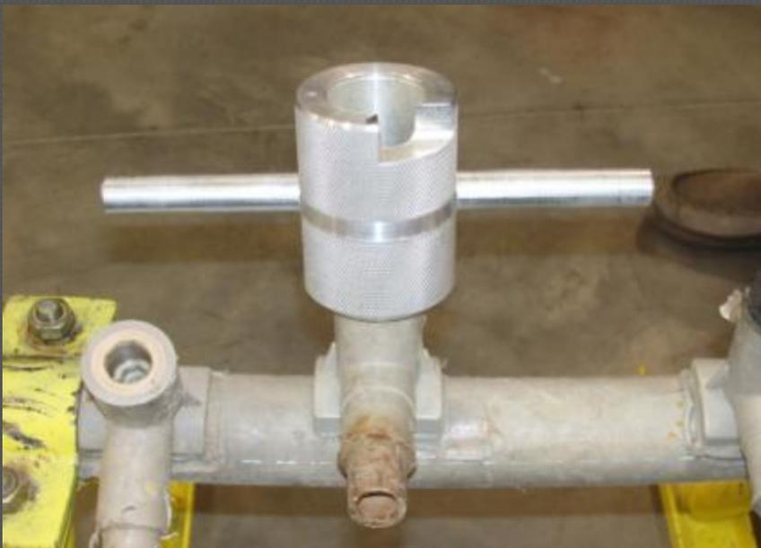
The outside diameter of the Aldyl-A tapping tee shall be scraped down to the intersection of the tee outlet.
