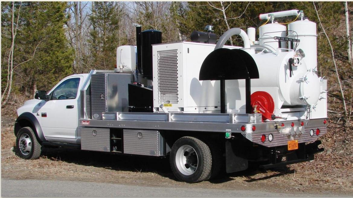
Gas evacuator systems can be used with any vacuum excavation that is equipped with a 4" diameter vacuum digging hose and has the ability to produce a flow rate from 780 to 1,100 SCFM.
