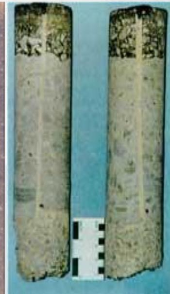
Cuts through kerf showing mechanical bond and no voids
