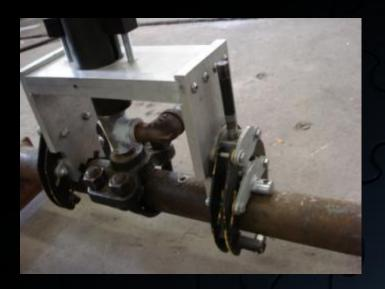
The "sealing chamber" provides a pressure tight connection between the pressure chamber and the live gas line.
