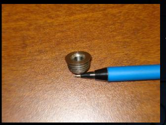
These plugs are designed to fit flush with the top of the main and have a small round protrusion into the inside of the main.
