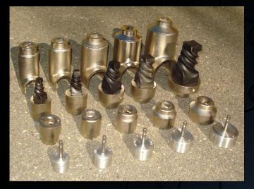
If the service tee breaks a specially designed "EZ Out" tool can be installed on the ¾" extension drive to remove the broken tee stub
