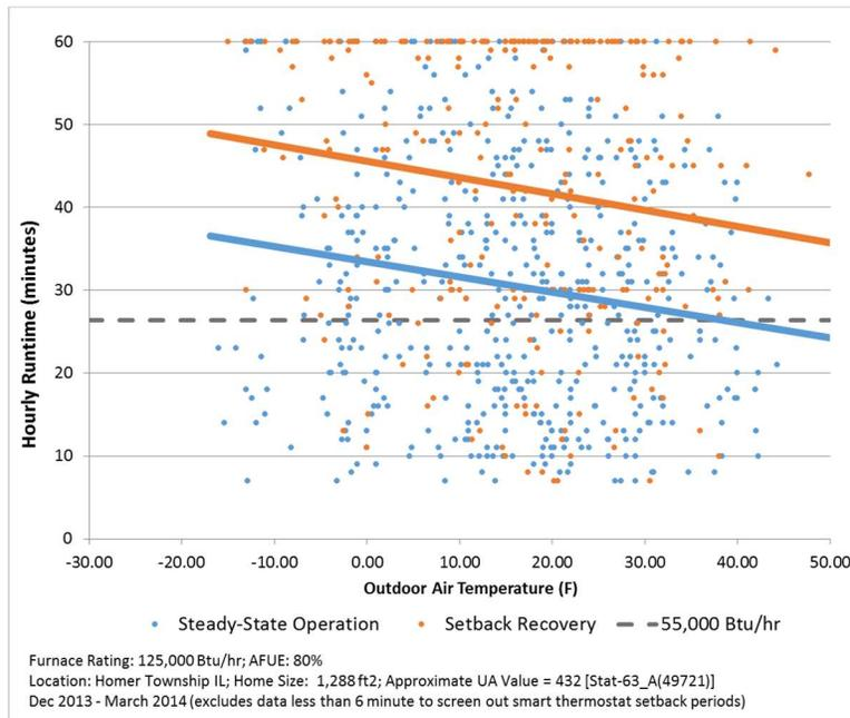
Figure 10: Example Furnace Steady-State and Setback Recovery Operation
