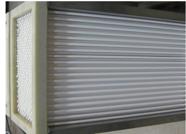
TMC tubes in a bundle assembly
