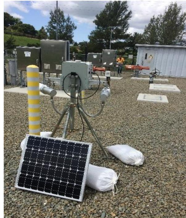
*Heath (right) and Sensit/Acutect (left) detectors installed at PG&E storage and regulation facilities*
