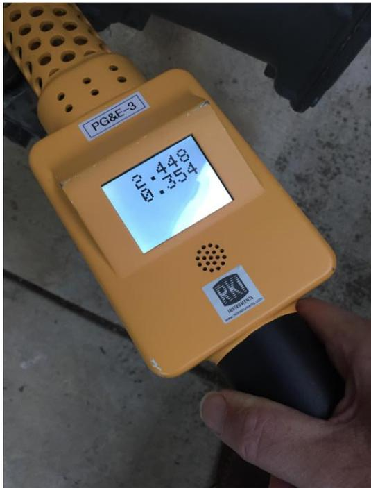
*Prototype of the handheld methane-ethane detector.*
