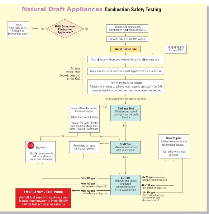
Fig. 5.9 Natural draft appliances - Mandatory combustion safety testing
