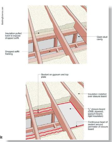
Fig. 9.4b Air sealing an open soffit
