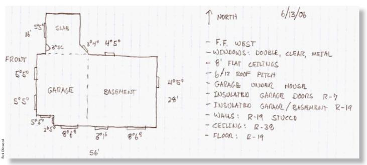
These days, such data is often recorded on tablet computers so it can be entered in load calculation programs directly. But hand sketches also work fine. Simply record the orientation of the building and dimensions of windows and walls—the key variables for heating & cooling loads.
