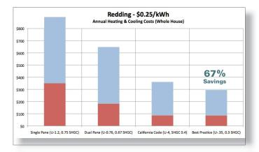
That said, it's possible to provide order-of-magnitude estimates which compare the effect of window choices on the whole house's annual heating & cooling costs in six California climates. These graphs show results for different costs of power—one which represents a current high-tier cost (24 e/kWh), and another (35 e/kWh) which may be common in the future. Other assumptions include:
