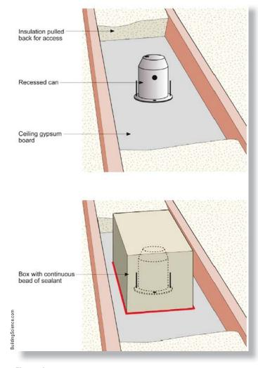
Fig. 9.11b Diagram of an insulated, air-tight cover for a can light
