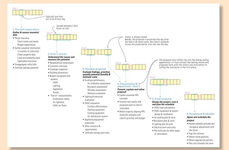
Fig. 3.1 Typical project development time line and tasks
