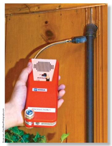
Fig. 5.13 Electronic gas leak detector - Audible indicator
