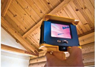
**Fig. 9.15 Thermal cameras can help locate less-obvious air leakage points** *Be careful, however, to choose a camera with adequate thermal sensitivity* (100 milliKevin or less, or less than 0.01°C).
