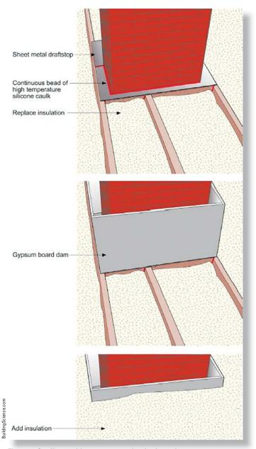
Fig. 9.8 Sealing a chimney penetration in the attic
