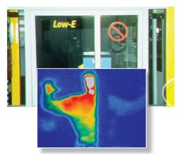
**Fig. 10.5 Low-E coatings also keep heat in the house during winter** *The thermal image shows how much more heat is reflected back into the house by the Low-E coating (the glass on the left) compared to the old-style uncoated glass on the right side of the same assembly.*
