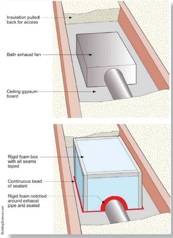
Fig. 9.12 Diagram of an insulated, air-tight cover for a leaky bathroom fan
