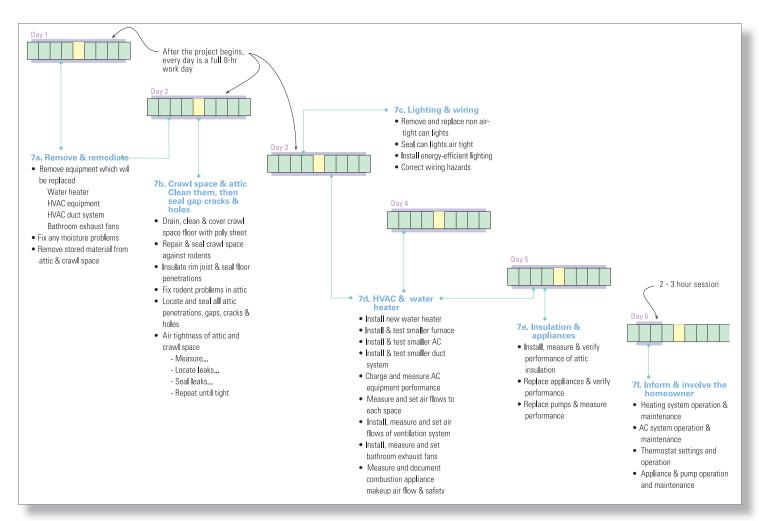
Fig. 3.6 Doing the work - Typical work sequence
