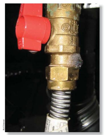
Fig. 5.14 Detergent solution - Visual gas leak detection
