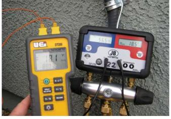
**Fig. 5.21 Semi-automatic superheat and subcooling calculations** Modern digital refrigerant guages calculate subcooling and superheat semi-automatically, based on temperature and pressure measurements and their built-in refrigerant property tables. This saves time and improves both accuracy and consistency of these critical measurements.
