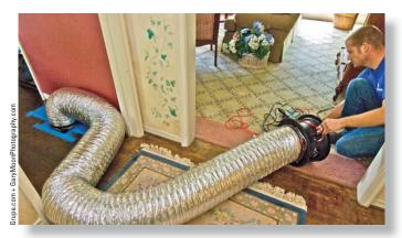
Fig. 5.19 Duct blaster, used in combination with the blower door for measuring duct leakage to the outdoors
